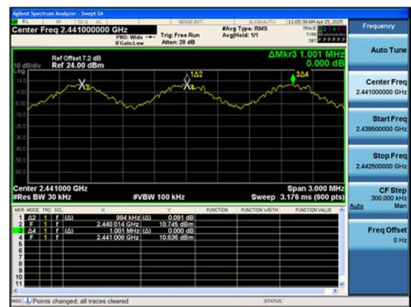
Dual ANT. 2 8DPSK : Channel Separation
