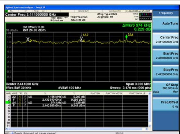
Dual ANT. 2 \pi/4 DQPSK : Channel Separation
