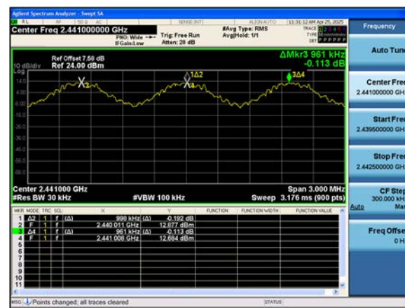
Dual ANT. 1 8DPSK : Channel Separation
