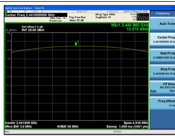
Dual ANT.2 8DPSK : Peak Power (Ch. 39)
