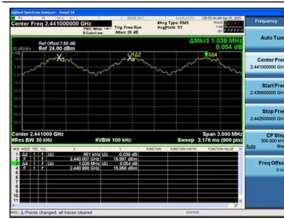
ANT. 1 8DPSK : Channel Separation
