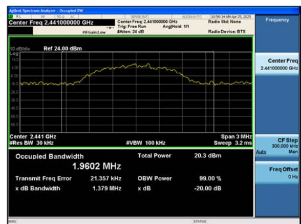
Dual ANT. 2 \pi/4 DQPSK 20 dB BW & 99% OBW (Ch. 0)
