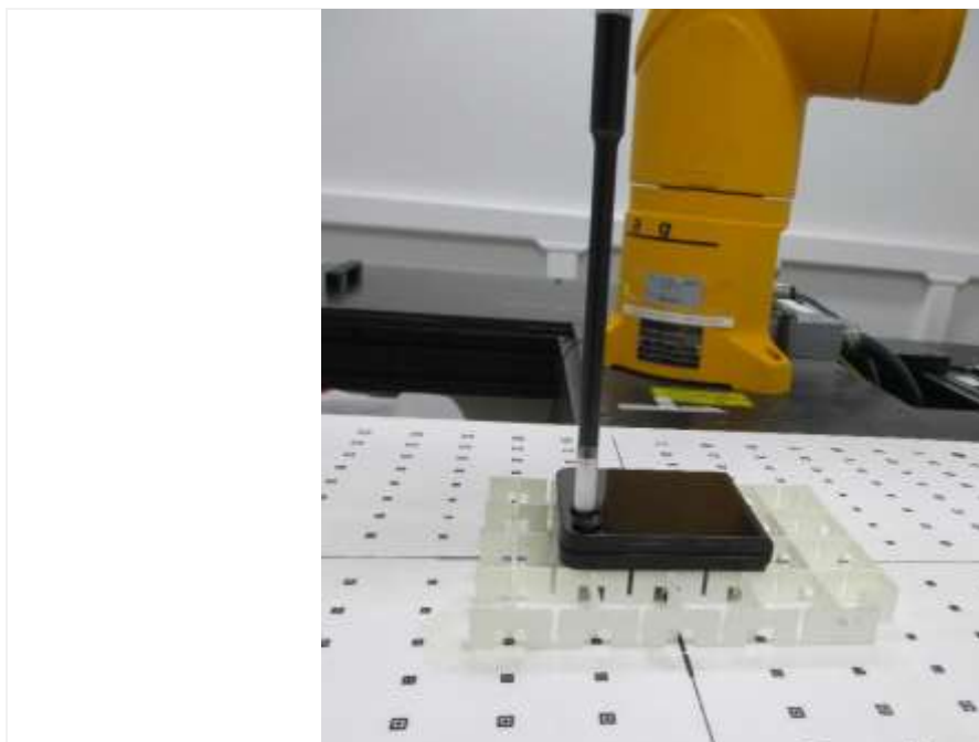
Distance of 2 mm from the EUT
