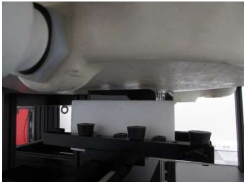
Distance of 5 mm from the EUT
