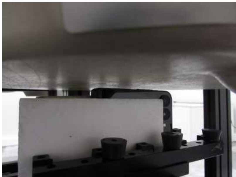
Distance of 5 mm from the EUT
