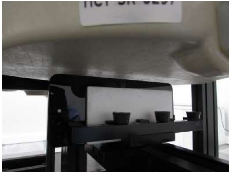
Distance of 5 mm from the EUT
