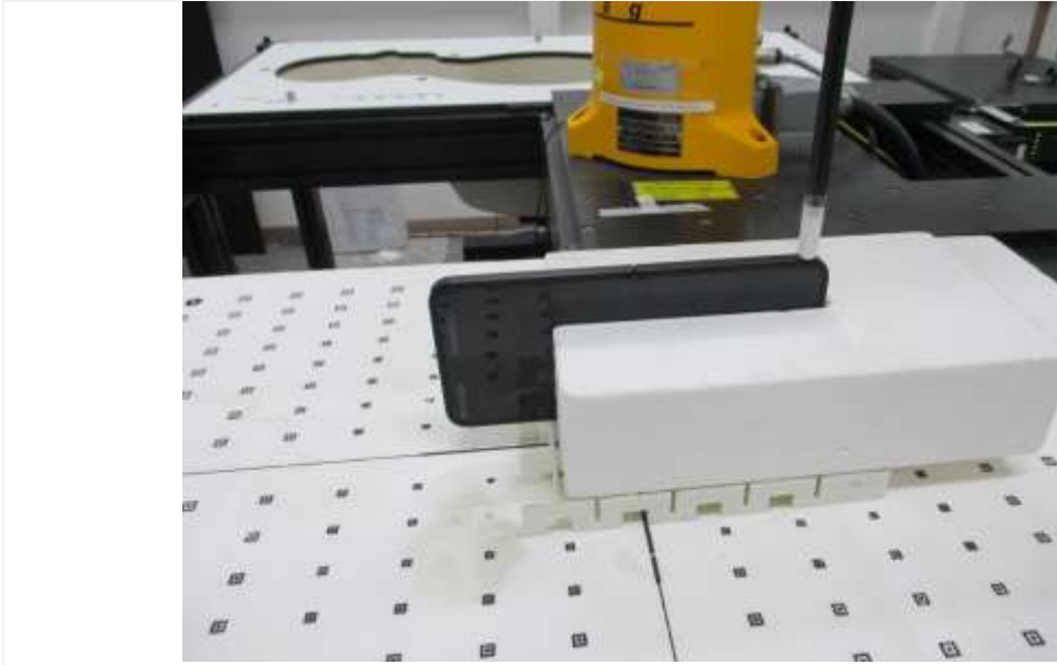
Distance of 2 mm from the EUT
