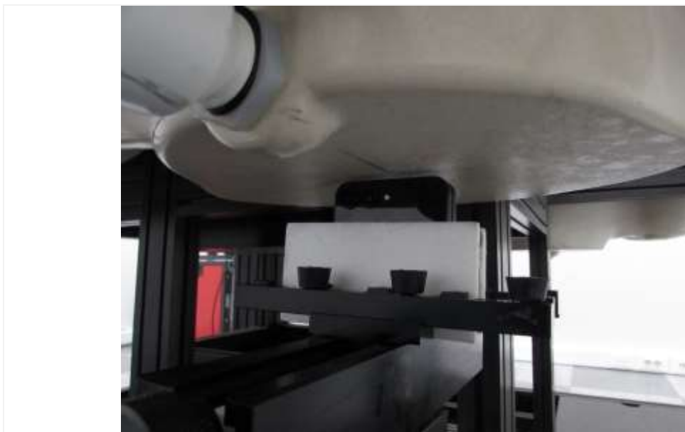
Distance of 5 mm from the EUT
