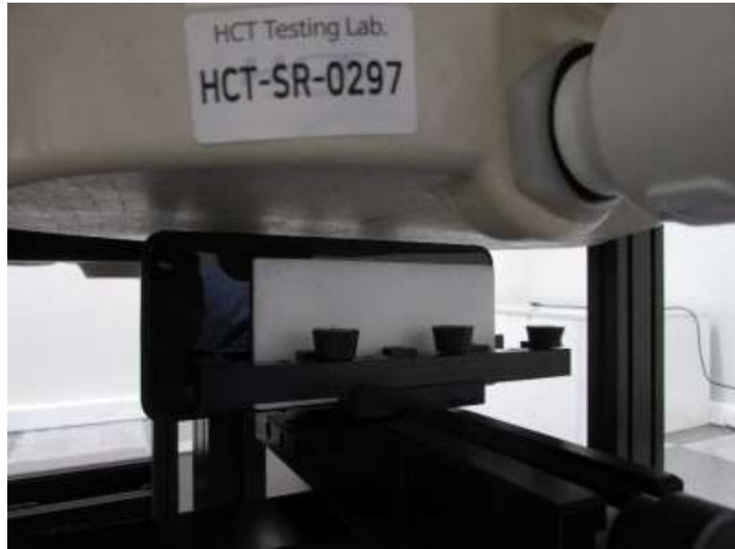
Distance of 5 mm from the EUT
