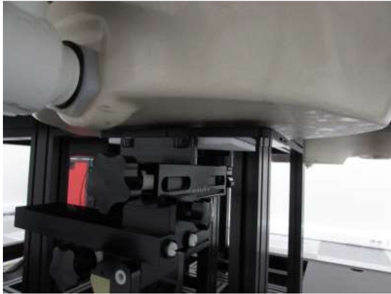
Distance of 5 mm from the EUT
