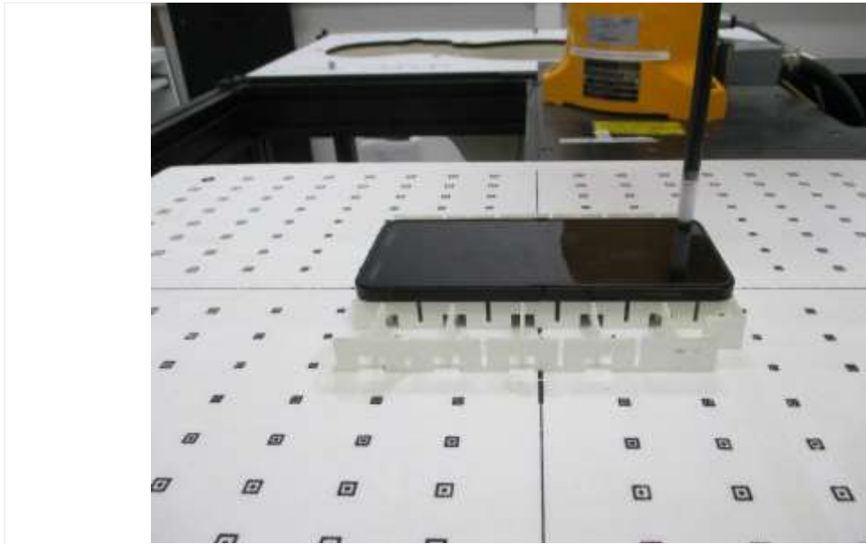
Distance of 2 mm from the EUT
