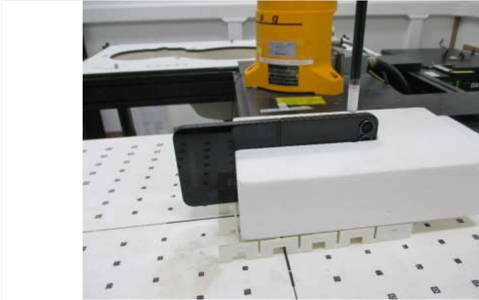
Distance of 2 mm from the EUT
