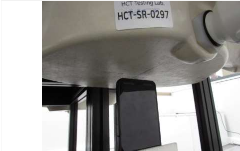
Distance of 5 mm from the EUT
