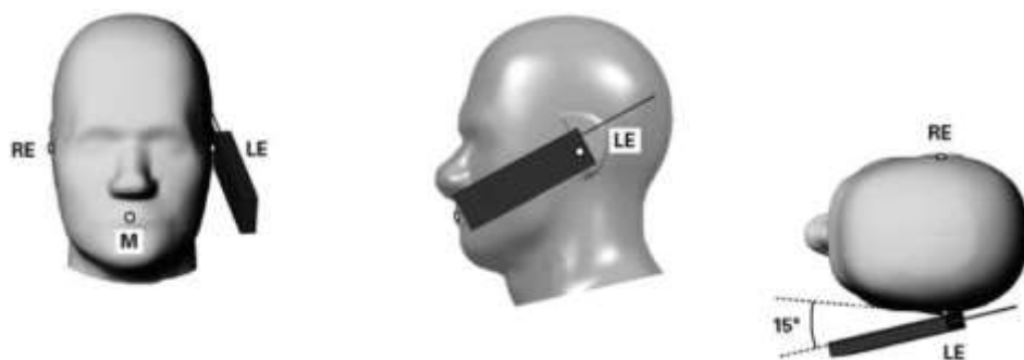
Figure 8.5. Tilt 15° position of the wireless device
