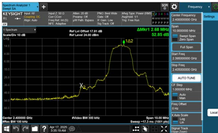
ANT.2 8DPSK Band Edge(Ch. 0)
