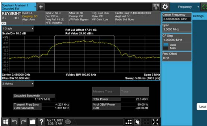
ANT. 1 \pi /4DQPSK 20 dB BW & 99% OBW (Ch. 39)
