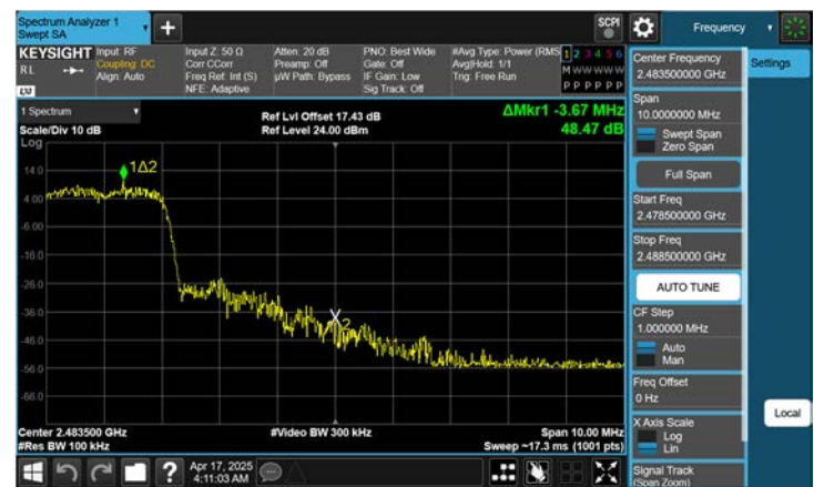
Dual ANT.2 \pi/4 DQPSK Band Edge(Ch. 78)
