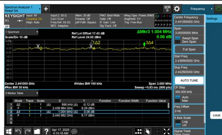
Dual ANT. 2\pi/4 DQPSK : Channel Separation
