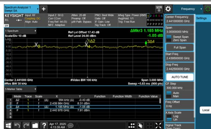
Dual ANT. 2\pi/4 DQPSK : Channel Separation
