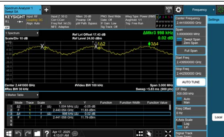
Dual ANT. 2 8DPSK: Channel Separation
