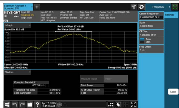
ANT. 2 8DPSK 20 dB BW & 99% OBW (Ch. 39)
