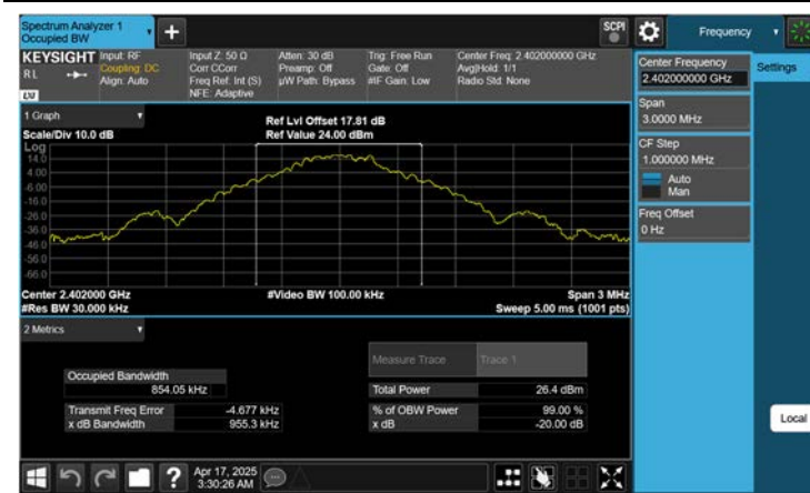
ANT. 1 8DPSK 20 dB BW & 99% OBW (Ch. 78)
