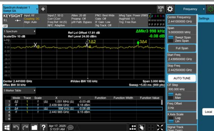
Dual ANT. 1 \pi/4 DQPSK: Channel Separation
