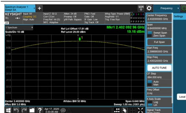
ANT.1 π/4DQPSK : Peak Power (Ch. 0)
