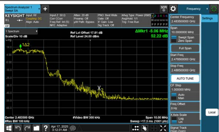
Dual ANT.2 \pi/4 DQPSK Band Edge(Ch. 78)
