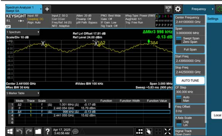
ANT. 1 8DPSK : Channel Separation
