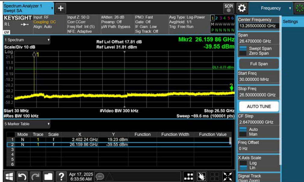
Spurious Emission (30 MHz - 26.50 GHz)Ant.2, GFSK Ch. 0
