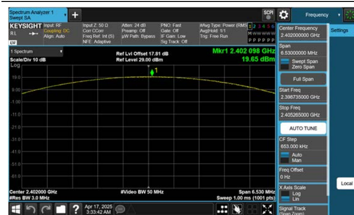
ANT.1 π/4DQPSK : Peak Power (Ch. 0)
