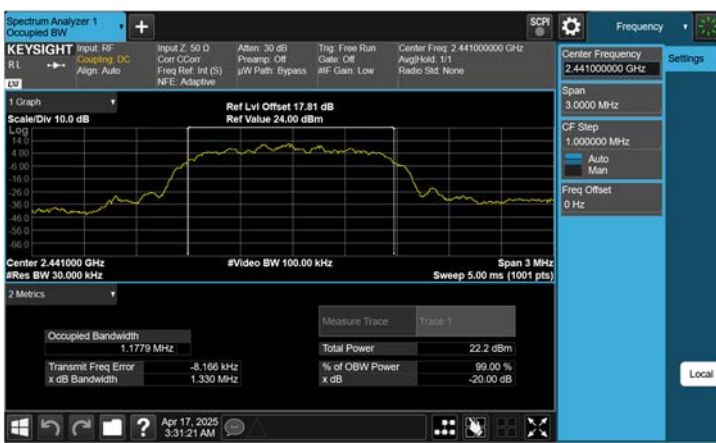
ANT. 1 \pi /4DQPSK 20 dB BW & 99% OBW (Ch. 39)
