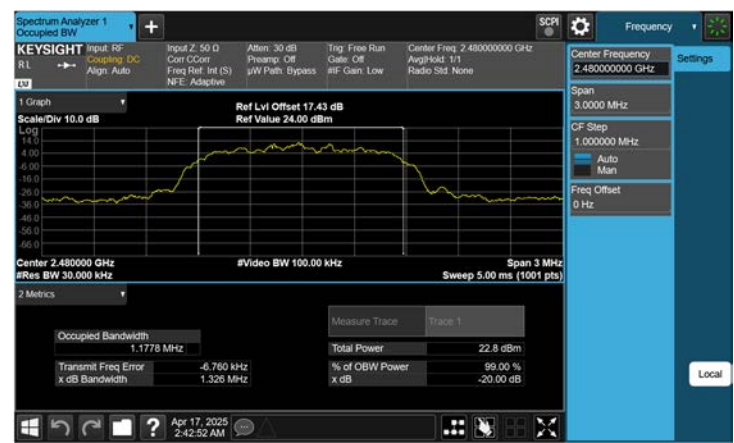
ANT. 2 \pi /4DQPSK 20 dB BW & 99% OBW (Ch. 78)
