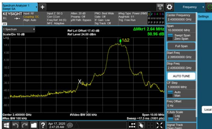
ANT.2 8DPSK Band Edge(Ch. 0)
