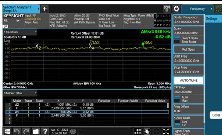
Dual ANT. 1 \pi/4 DQPSK: Channel Separation
