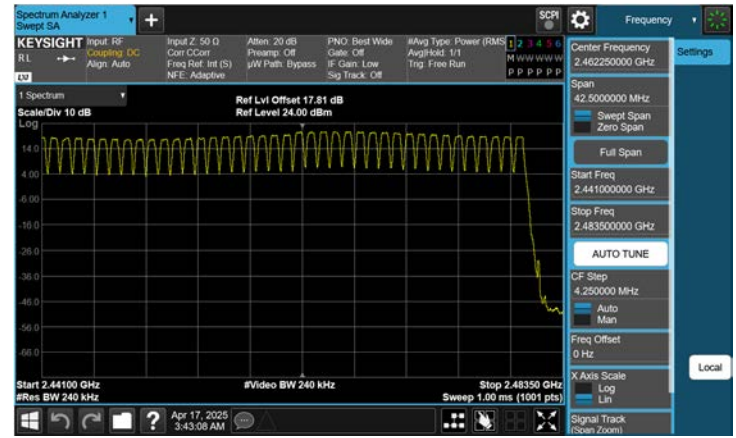
ANT.1 8DPSK (2.441 GHz - 2.483.5 GHz)
