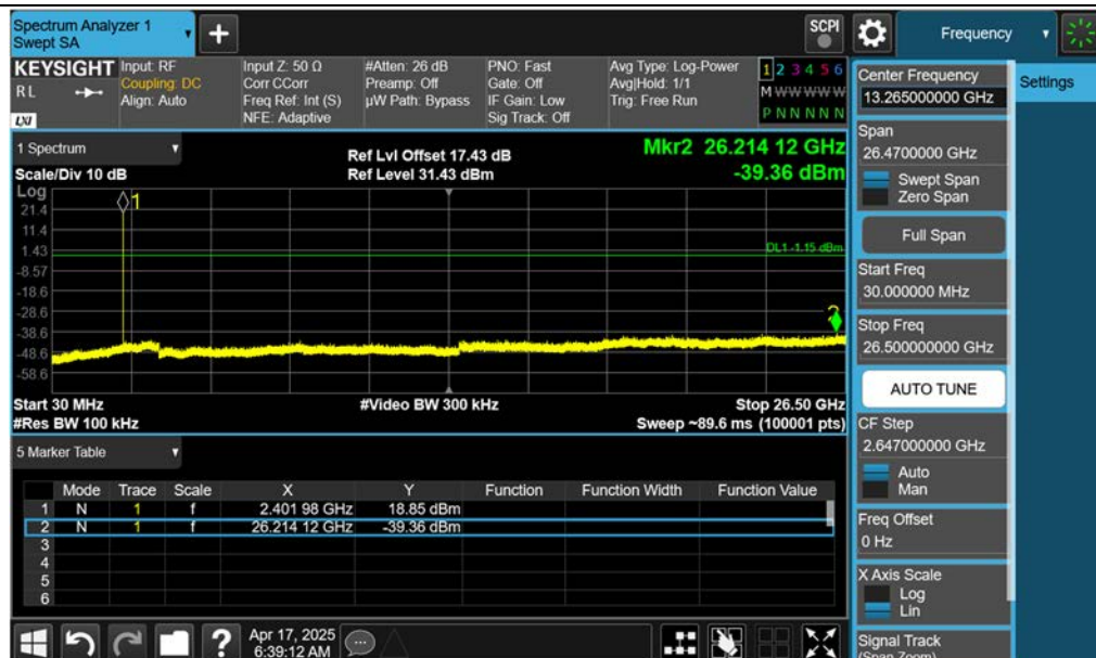
Spurious Emission (30 MHz - 26.50 GHz)Ant.2, GFSK Ch. 0
