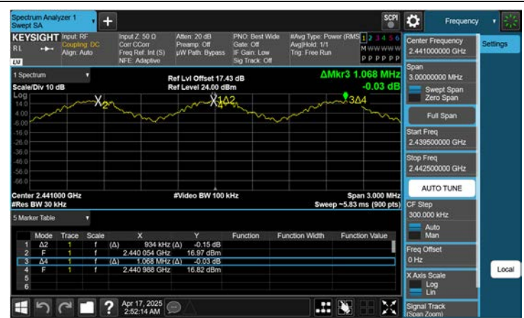
ANT. 2 8DPSK : Channel Separation
