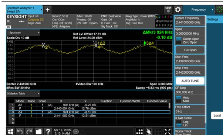
Dual ANT. 18DPSK: Channel Separation
