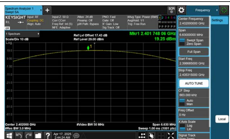
ANT.2 π/4DQPSK : Peak Power (Ch. 0)
