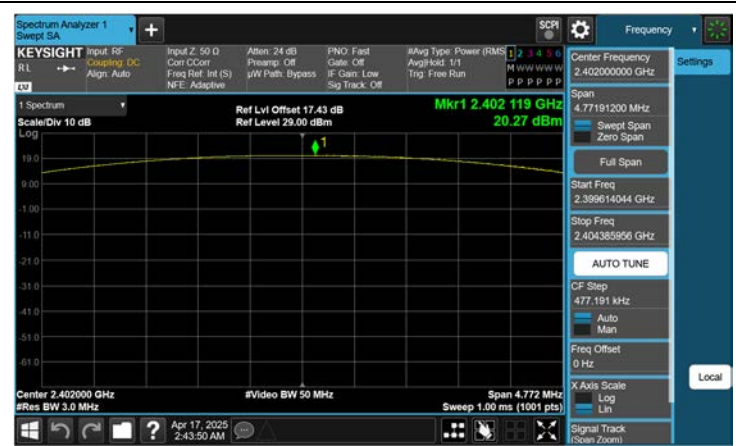
ANT.2 8DPSK : Peak Power (Ch. 0)
