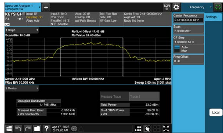
ANT. 2 \pi /4DQPSK 20 dB BW & 99% OBW (Ch. 78)
