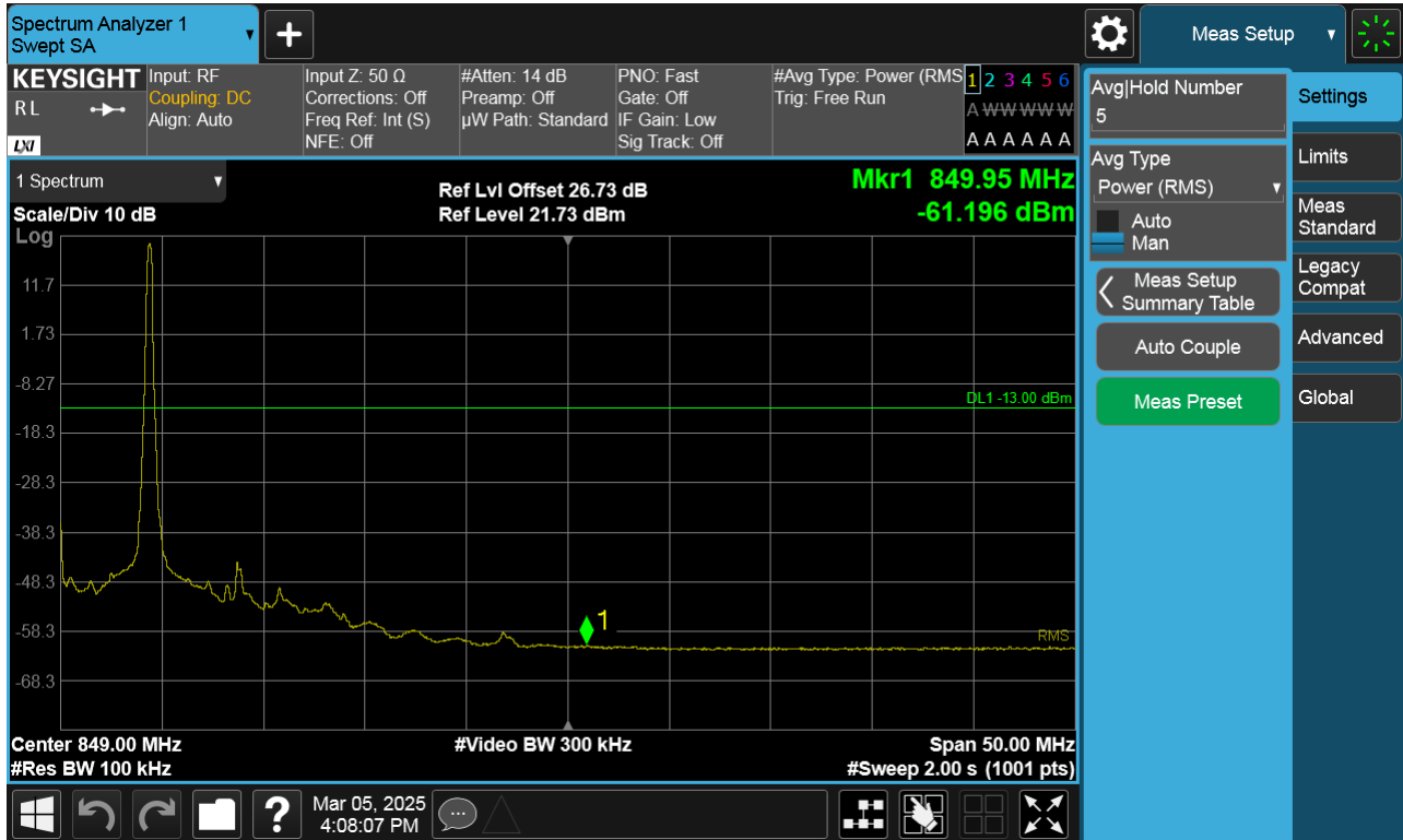
Sub6 n26. Upper Band Edge Plot (10 M BW Ch.164800 BPSK_RB1_Offset 51)
