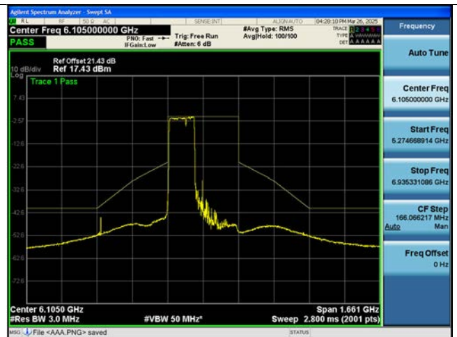
Bandwidth 320M, Ch. 31(6105 MHz) 996T+484T RU1095
