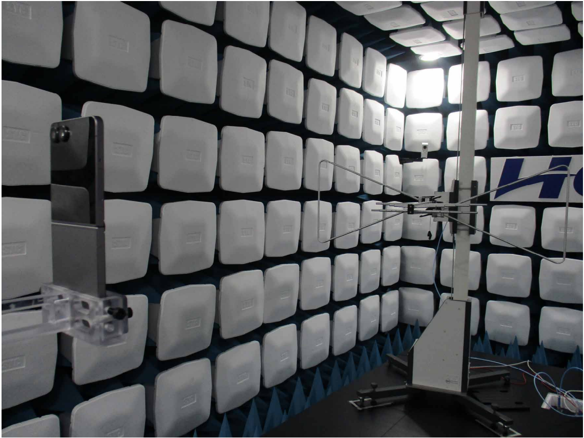
2. Radiated Test Setup Photo(mmW)
