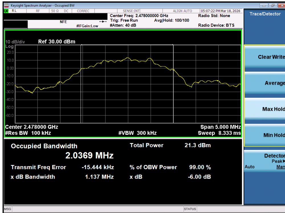
Plot 7-30. 6dB Bandwidth Plot (Bluetooth (LE), 2Mbps – Ch. 36) – Dual Ant 1
