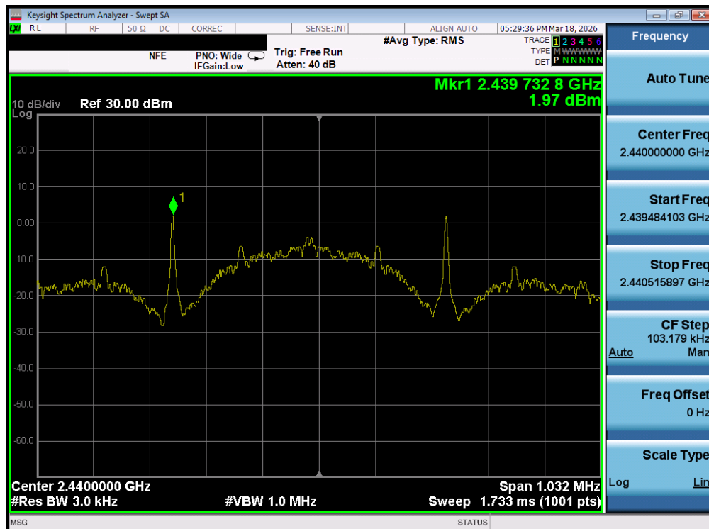
Plot 7-86. Power Spectral Density Plot (Bluetooth (LE), 125kbps – Ch. 17) – Ant 2
