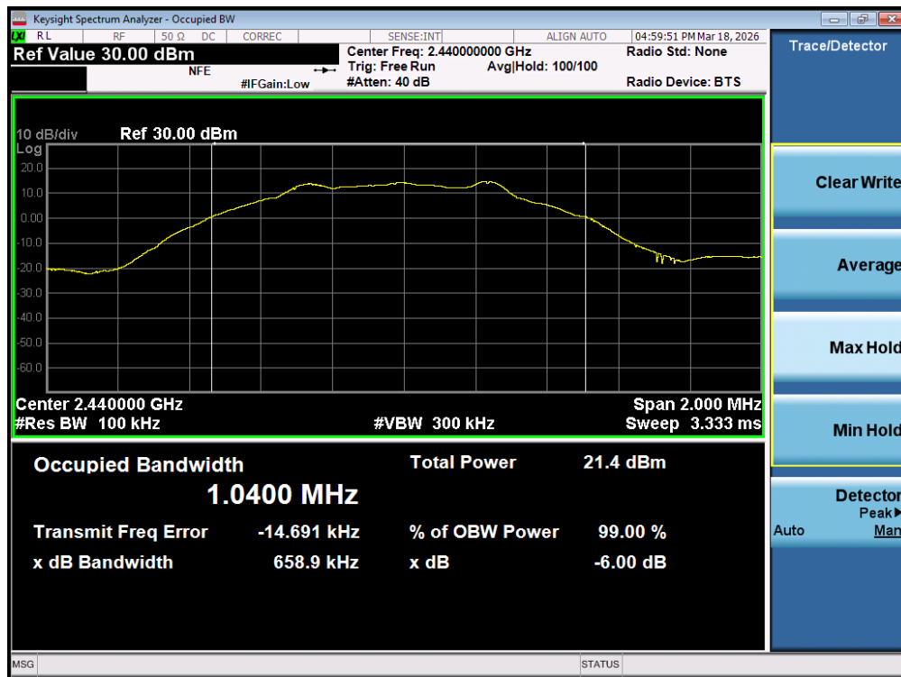
Plot 7-26. 6dB Bandwidth Plot (Bluetooth (LE), 1Mbps – Ch. 17) – Dual Ant 1
