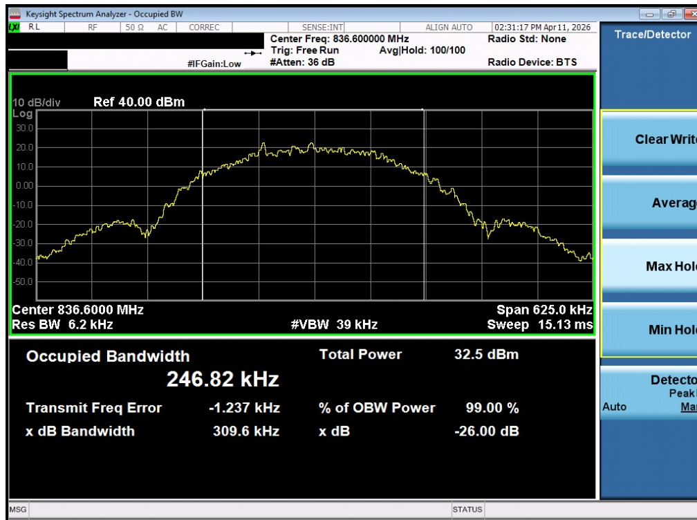
Plot 7-2. Occupied Bandwidth Plot (EDGE, Ch. 190 – Ant1)
