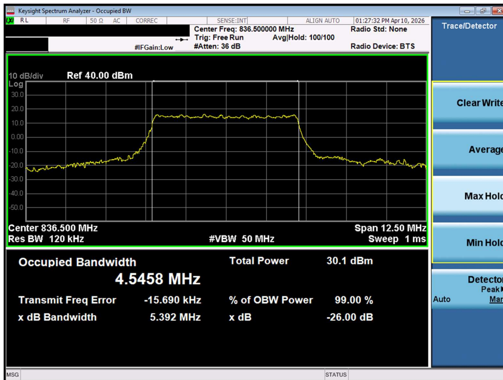
Plot 7-25. Occupied Bandwidth Plot (NR Band n5 - 5MHz 16-QAM - Full RB - Ant1)
