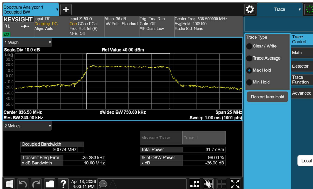
Plot 7-32. Occupied Bandwidth Plot (LTE Band 26/5 - 10MHz 16-QAM - Full RB – Ant2)
