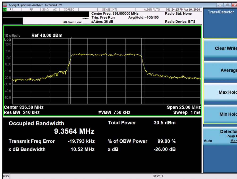
Plot 7-21. Occupied Bandwidth Plot (NR Band n5 - 10MHz QPSK - Full RB - Ant1)
