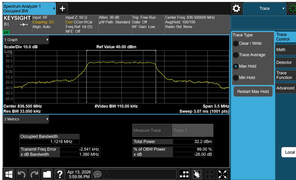
Plot 7-37. Occupied Bandwidth Plot (LTE Band 26/5 – 1.4MHz QPSK - Full RB – Ant2)
