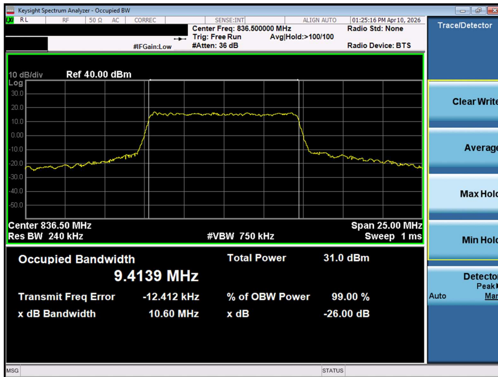
Plot 7-22. Occupied Bandwidth Plot (NR Band n5 - 10MHz 16-QAM - Full RB - Ant1)
