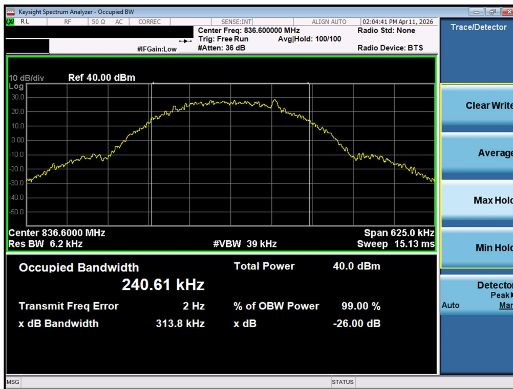
Plot 7-26. Occupied Bandwidth Plot (GPRS, Ch. 190 – Ant2)
