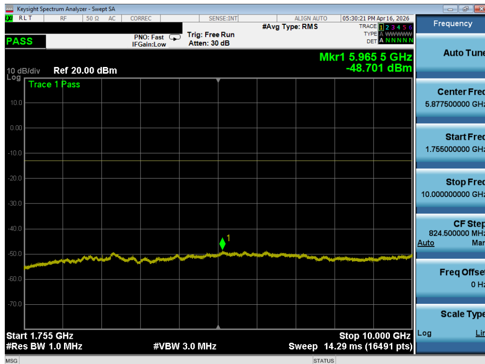
Plot 7-136. Conducted Spurious Plot (WCDMA-AWS - 5MHz QPSK - 1 RB – Low Channel – ANT2)
