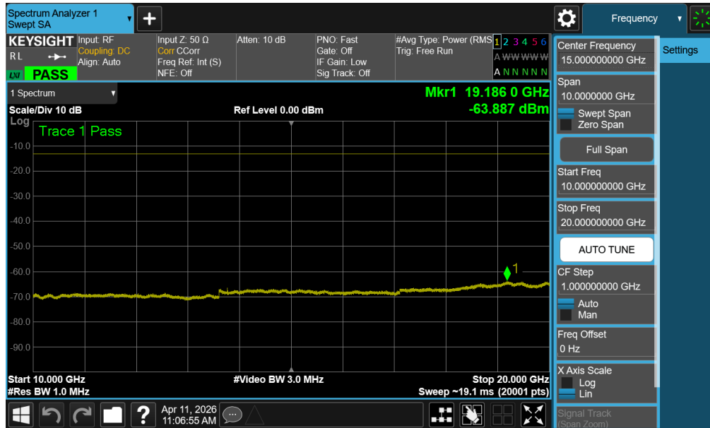
Plot 7-131. Conducted Spurious Plot (LTE Band 66/4 - 20MHz QPSK - 1 RB – Low Channel)
