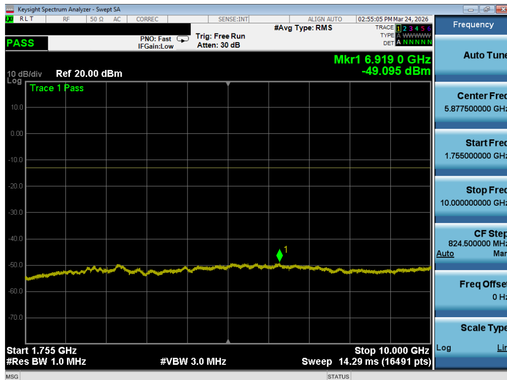
Plot 7-118. Conducted Spurious Plot (WCDMA-AWS – Low Channel)
