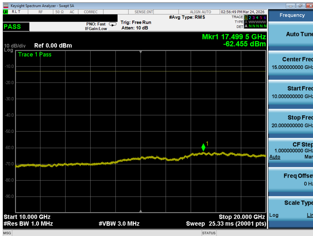
Plot 7-119. Conducted Spurious Plot (WCDMA-AWS – Low Channel)
