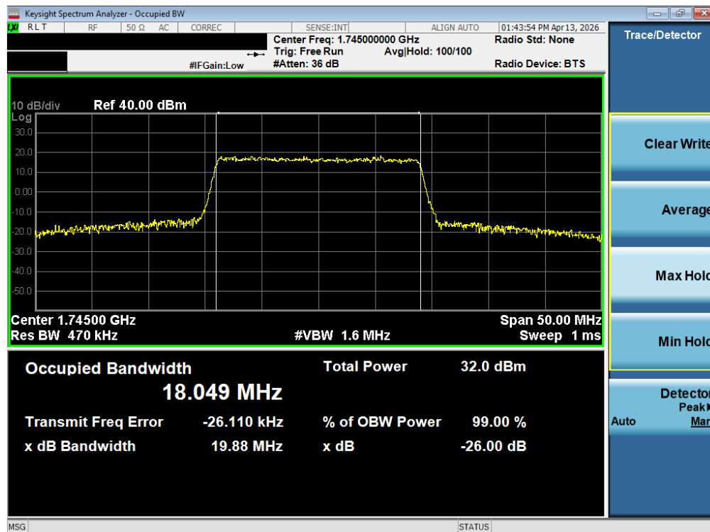
Plot 7-73. Occupied Bandwidth Plot (LTE Band 66/4 - 20MHz 16-QAM - Full RB - ANT2)
