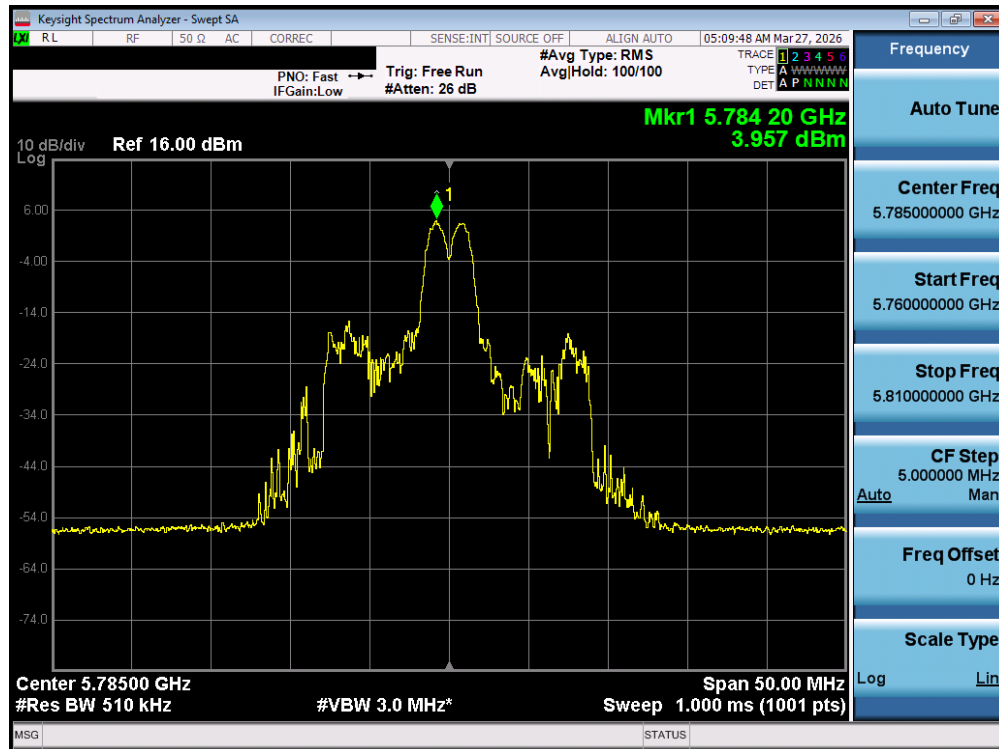
Plot 7-65. Power Spectral Density Plot MIMO ANT1 (20MHz BW 802.11be – 26 Tones (UNII Band 3) – Ch. 157)
