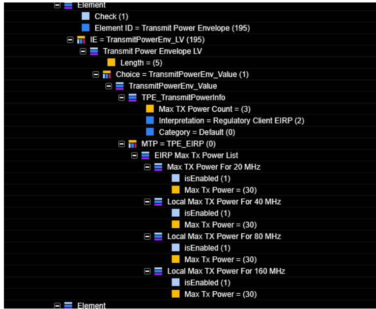
Figure 7-9. Callbox Power Authorization – 21.00dBm
