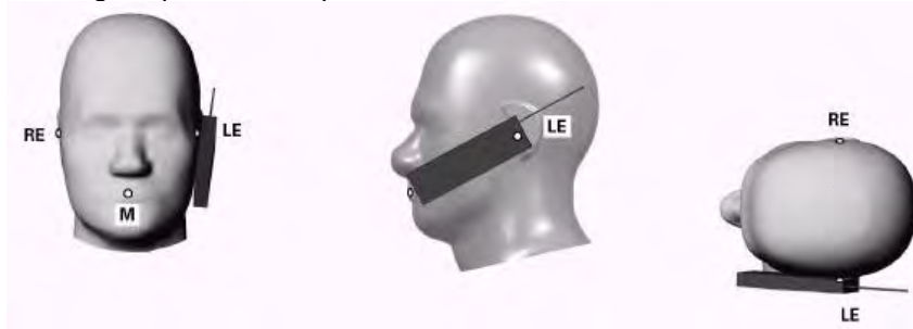
Figure 7-1 Front, Side and Top View of Cheek Position
