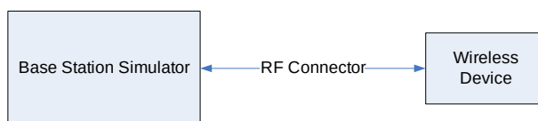
Figure 10-4 Power Measurement Setup – NR FDD
