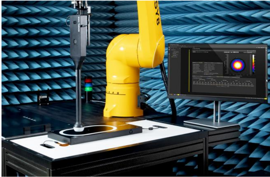
Figure 3-1 DASY 6/8 Module WPT V2.6+ Test System
