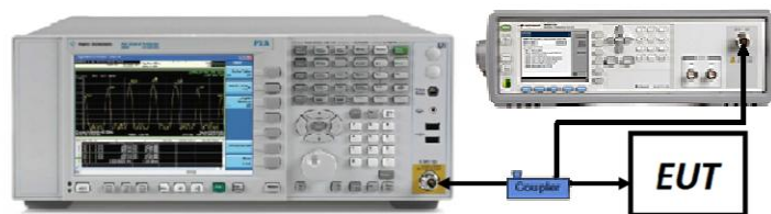
Figure 7-6. Test Instrument & Measurement Setup
