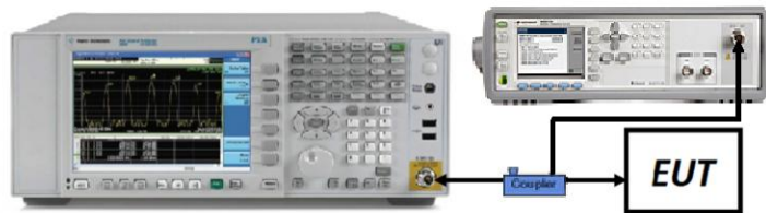
Figure 7-7. Test Instrument & Measurement Setup
