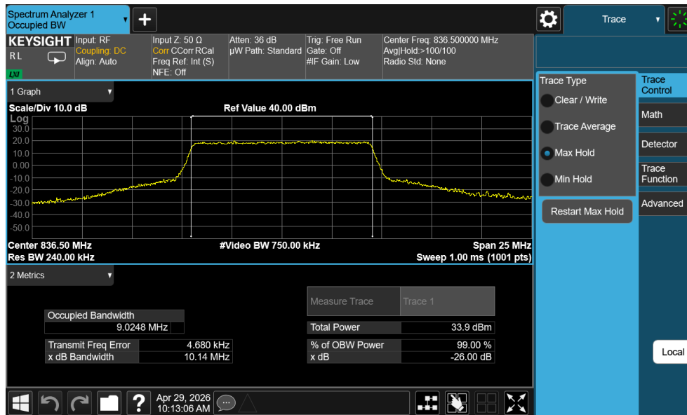
Plot 9-3. Occupied Bandwidth (Spot-check) – LTE Band5 (Spot-check)
