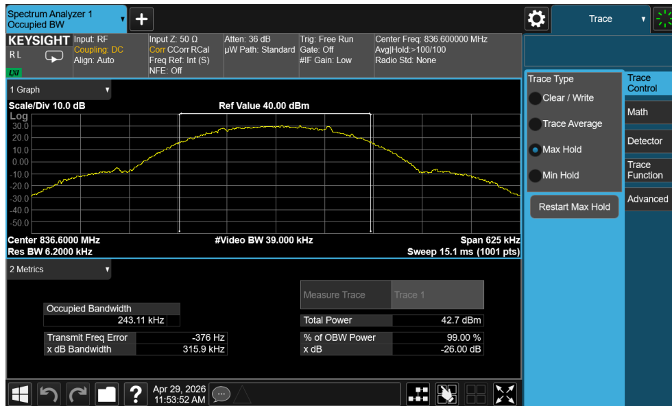
Plot 9-1. Occupied Bandwidth (Spot-check) – GPRS850 (Spot-check)
