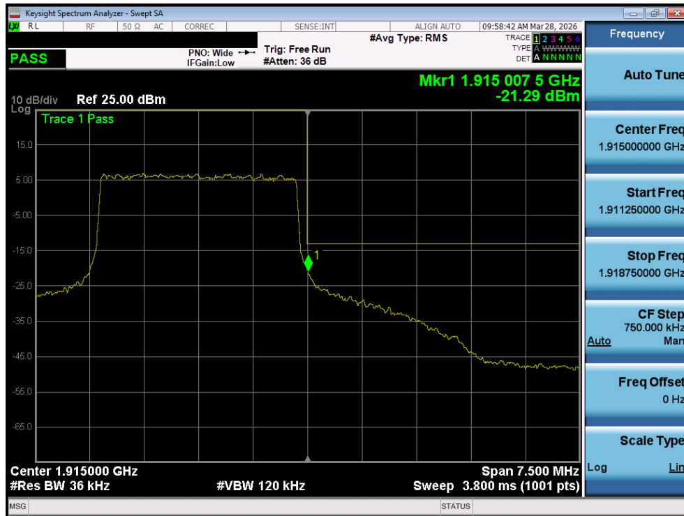
Plot 7-48. Upper Band Edge Plot (LTE Band 25 - 3MHz QPSK - Full RB - Ant2)
