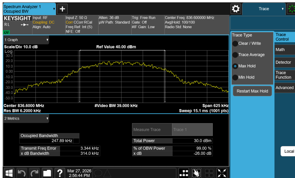
Plot 7-2. Occupied Bandwidth Plot (EDGE, Ch. 661 – Ant1)
