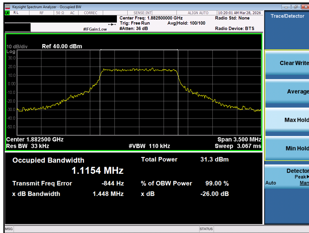
Plot 7-14. Occupied Bandwidth Plot (LTE Band 25/2 - 1.4MHz 16-QAM - Full RB - Ant1)
