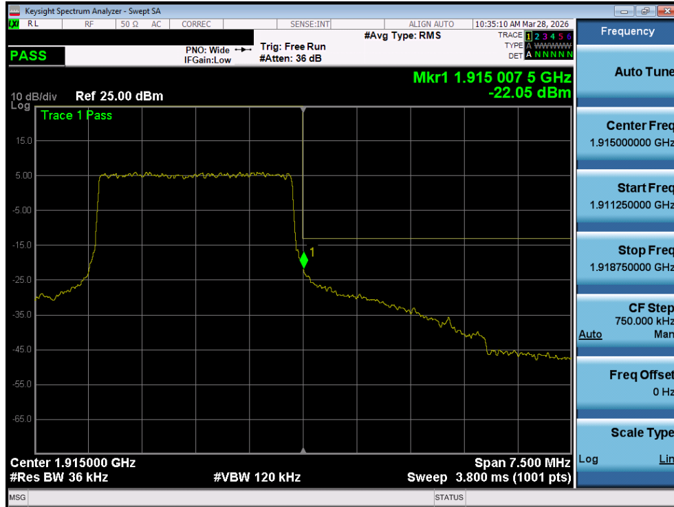
Plot 7-42. Upper Band Edge Plot (LTE Band 25 – 3MHz QPSK – Full RB - Ant1)
