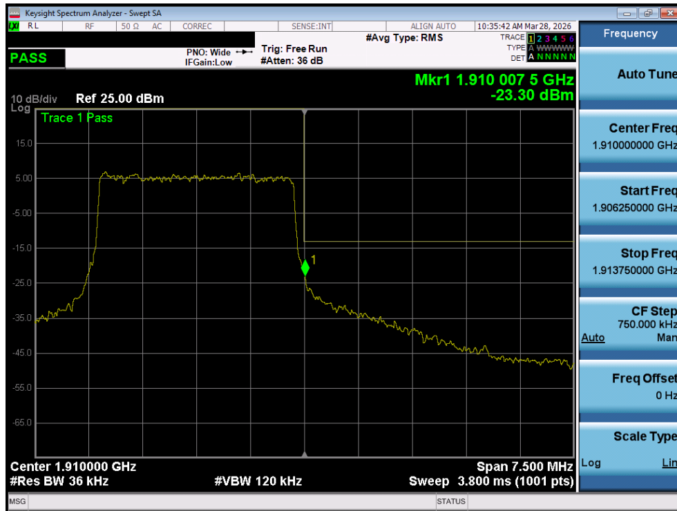
Plot 7-40. Upper Band Edge Plot (LTE Band 2 - 3MHz QPSK - Full RB - Ant1)
