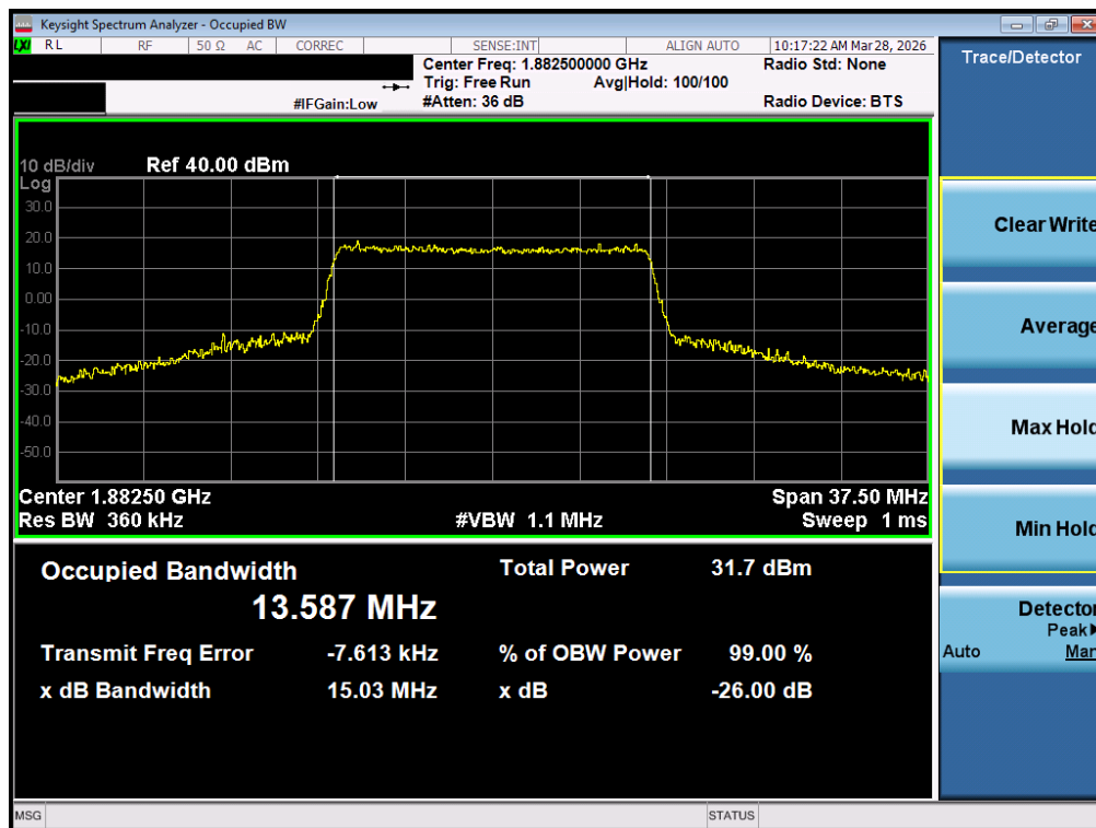
Plot 7-6. Occupied Bandwidth Plot (LTE Band 25/2 - 15MHz 16-QAM - Full RB - Ant1)
