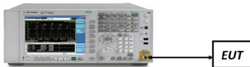
Figure 7-4. Test Instrument & Measurement Setup
