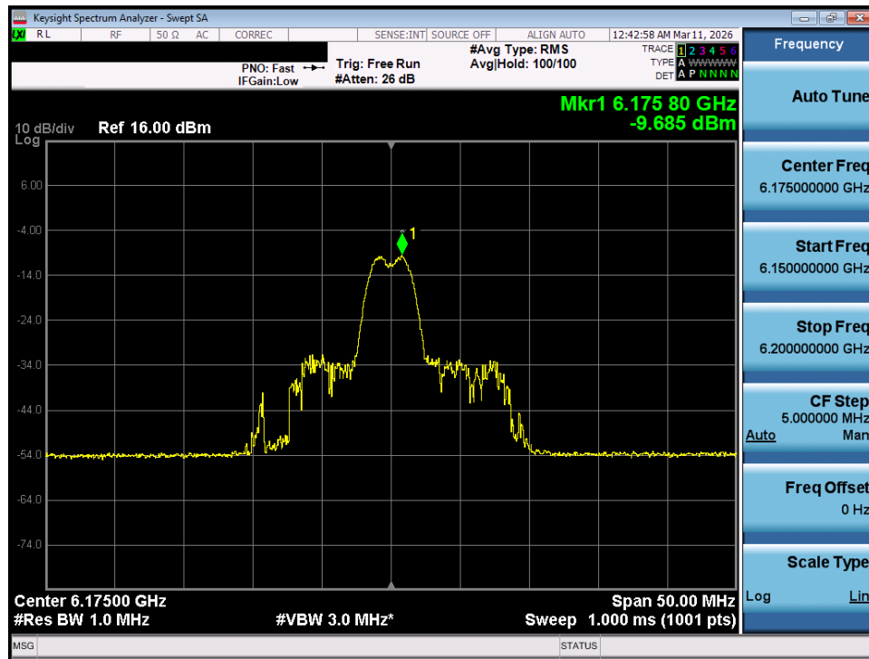
Plot 7-29. Power Spectral Density Plot MIMO ANT1 (20MHz 802.11ax/be (26 Tones) (UNII Band 5) – Ch. 45) - VLP
