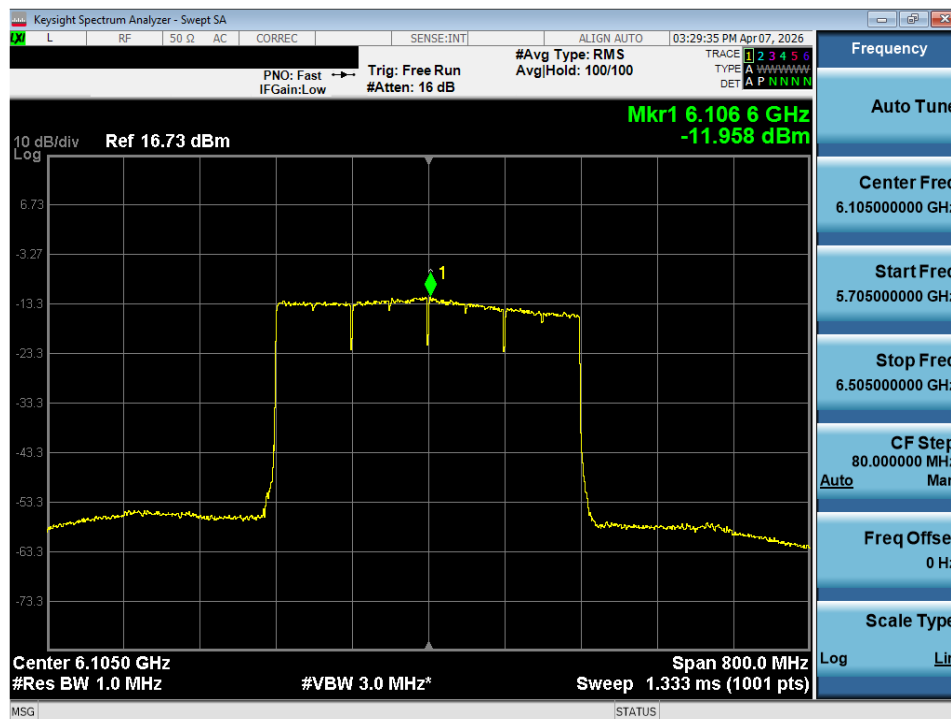
Plot 7-56. Power Spectral Density Plot MIMO ANT2 (320MHz 802.11be (Full Tones) (UNII Band 5) – Ch. 31) - VLP
