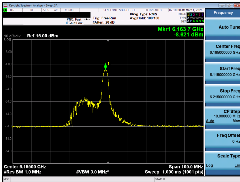
Plot 7-30. Power Spectral Density Plot MIMO ANT1 (40MHz 802.11ax/be (26 Tones) (UNII Band 5) – Ch. 43) - VLP
