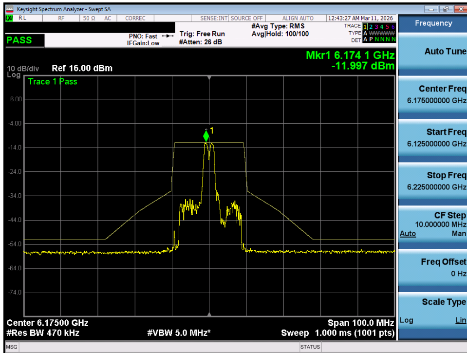
Plot 7-57. In Band Emissions Plot MIMO ANT1 (20MHz 802.11ax/be (26 Tones) (UNII Band 5) – Ch. 45) - VLP
