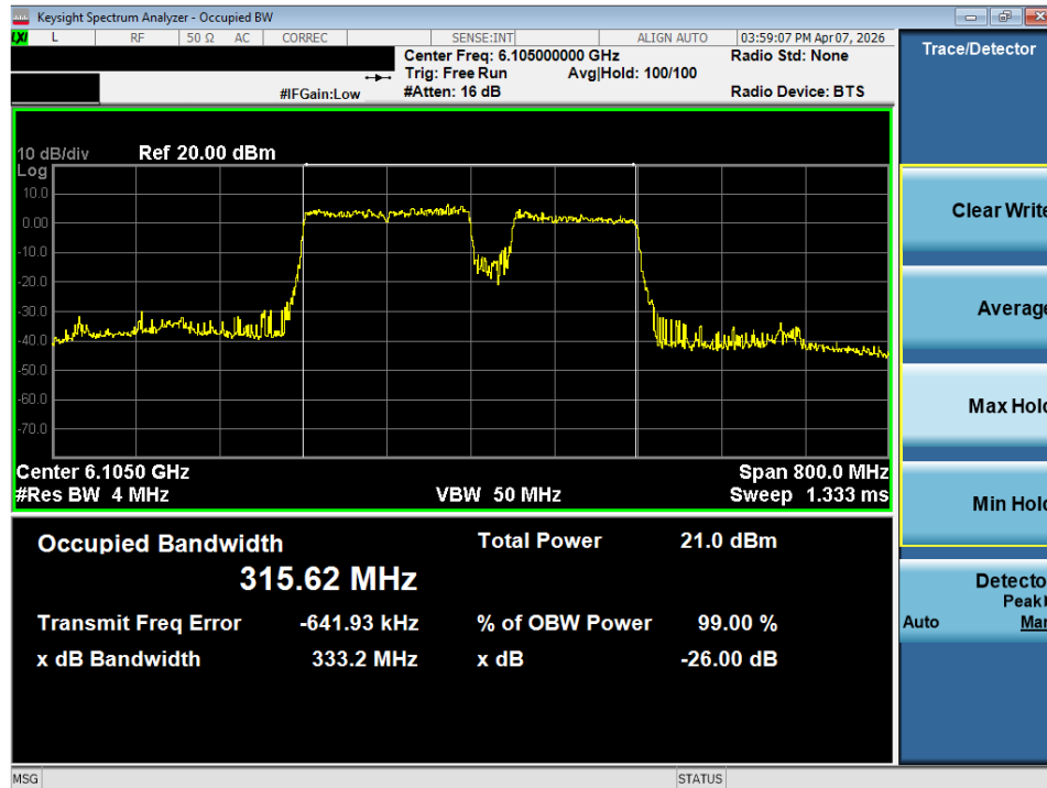
Plot 7-23. 26dB Bandwidth Plot MIMO ANT2 (320MHz 802.11be (3*996+484 Tones) (UNII Band 5) – Ch. 31) VLP
