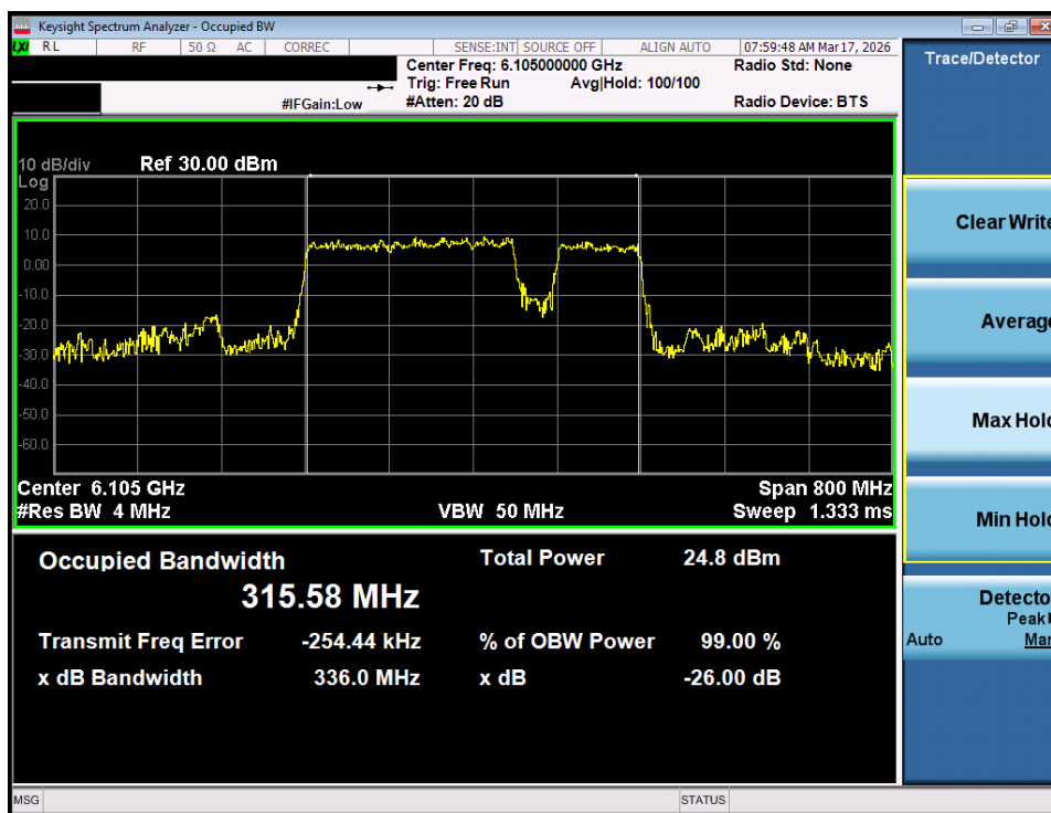
Plot 7-9. 26dB Bandwidth Plot MIMO ANT1 (320MHz 802.11be (3*996+484 Tones) (UNII Band 5) – Ch. 31) LPI/SP
