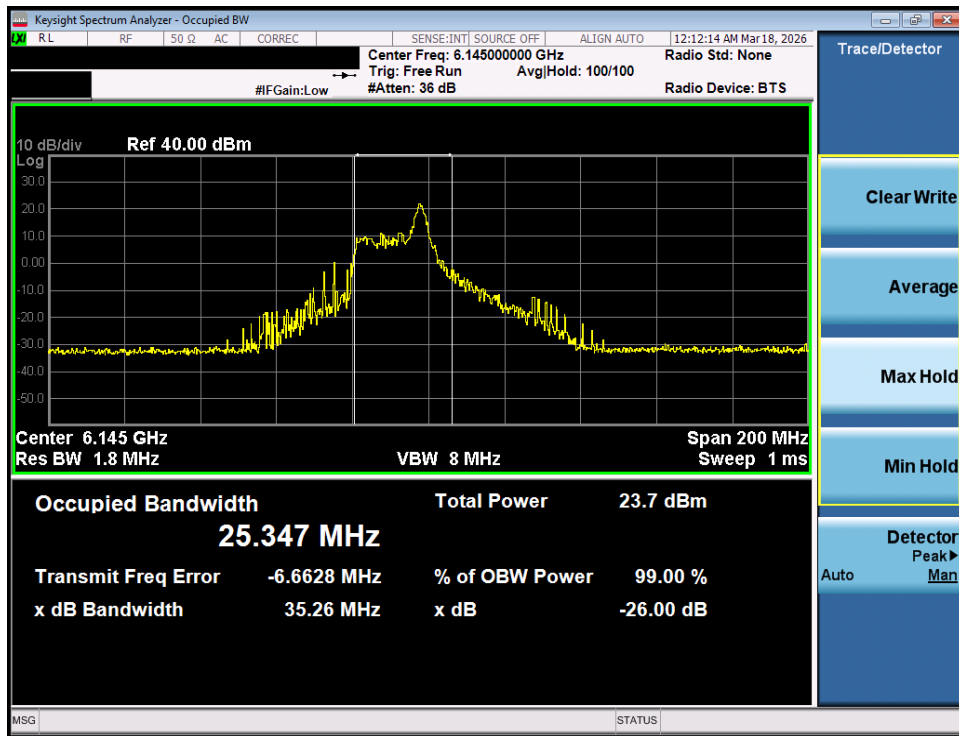
Plot 7-12. 26dB Bandwidth Plot MIMO ANT1 (80MHz 802.11ax/be (26 Tones) (UNII Band 5) – Ch. 39) - SP
