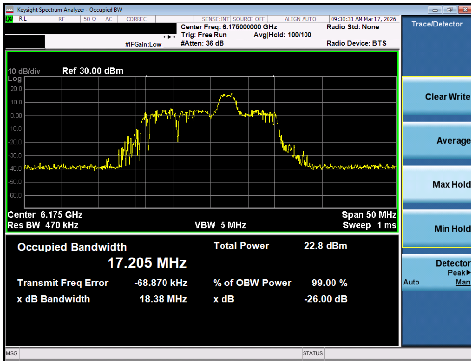
Plot 7-10. 26dB Bandwidth Plot MIMO ANT1 (20MHz 802.11ax/be (26 Tones) (UNII Band 5) – Ch. 45) – SP
