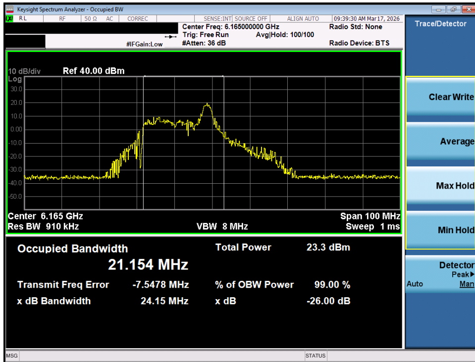
Plot 7-11. 26dB Bandwidth Plot MIMO ANT1 (40MHz 802.11ax/be (26 Tones) (UNII Band 5) – Ch. 43) - SP
