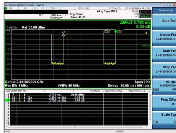
Figure 10-8 Bluetooth Antenna G Transmission Plot
