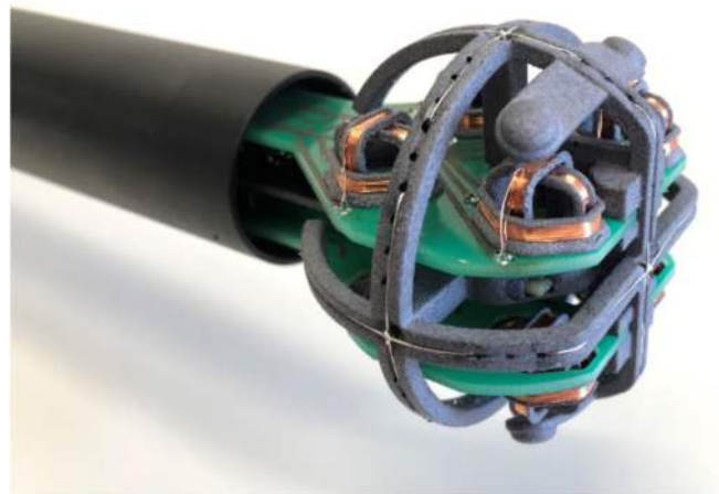
Figure 2-2 MAGPy-8H3D+E3 V2 Measurement Probe
