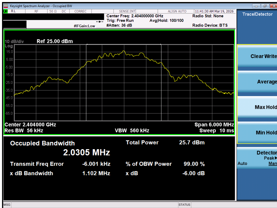
Plot 7-46. OBW Plot (Bluetooth (LE), 2Mbps – Ch. 0) – SISO ANT1
