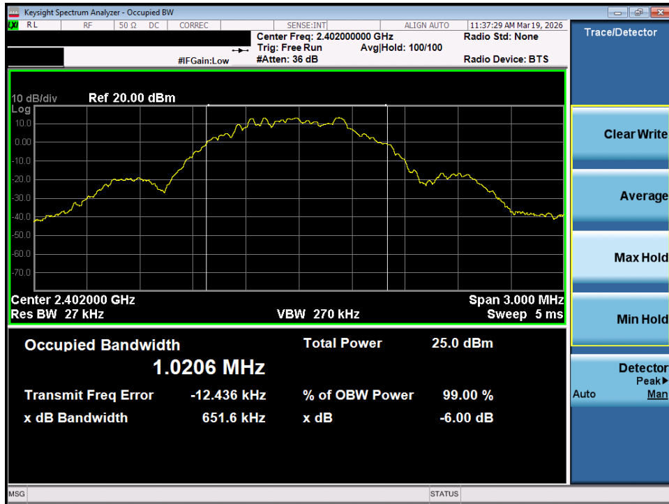
Plot 7-43. OBW Plot (Bluetooth (LE), 1Mbps – Ch. 37) – SISO ANT1
