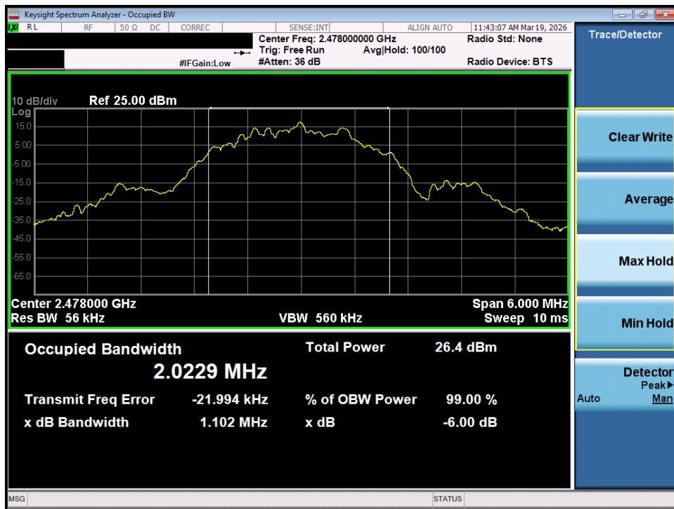
Plot 7-48. OBW Plot (Bluetooth (LE), 2Mbps – Ch. 36) – SISO ANT1
