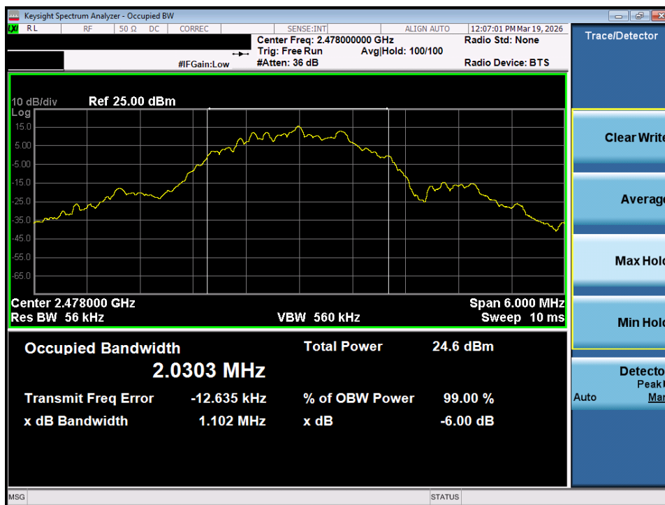
Plot 7-60. OBW Plot (Bluetooth (LE), 2Mbps – Ch. 36) – SISO ANT2
