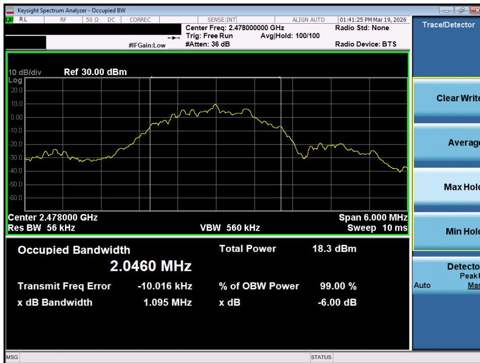
Plot 7-72. OBW Plot (Bluetooth (LE), 2Mbps – Ch. 36) – Dual ANT2
