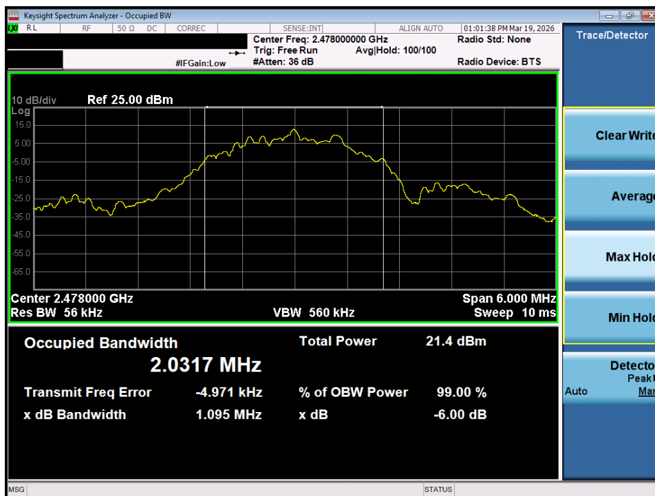
Plot 7-66. OBW Plot (Bluetooth (LE), 2Mbps - Ch. 36) - Dual ANT1
