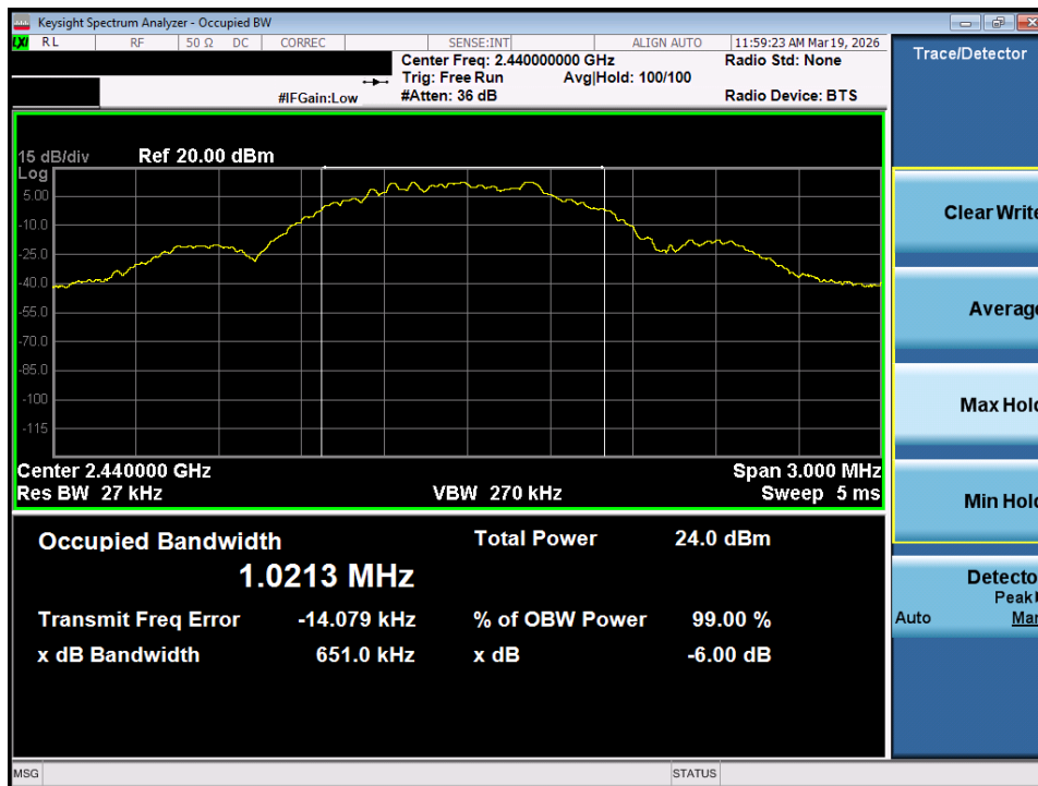
Plot 7-56. OBW Plot (Bluetooth (LE), 1Mbps – Ch. 17) – SISO ANT2
