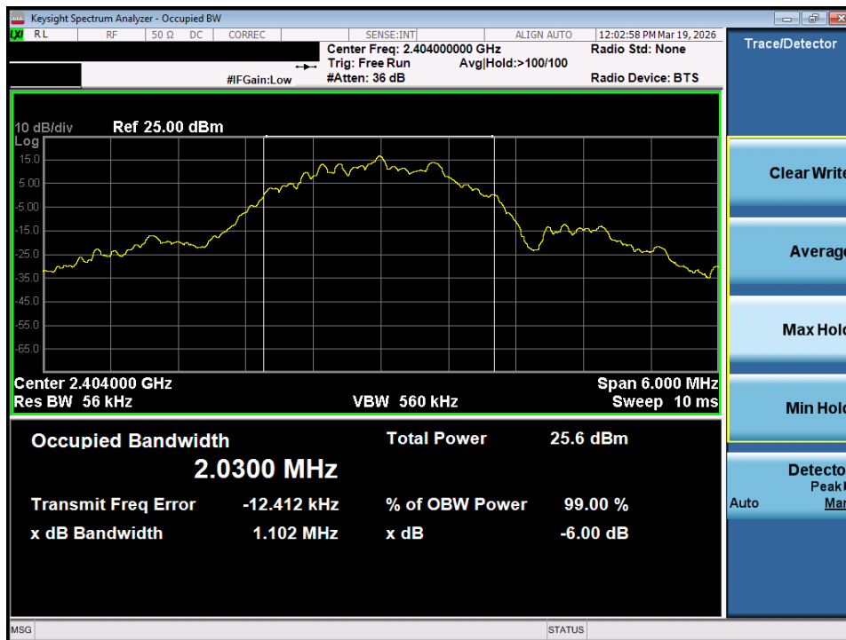
Plot 7-58. OBW Plot (Bluetooth (LE), 2Mbps – Ch. 0) – SISO ANT2
