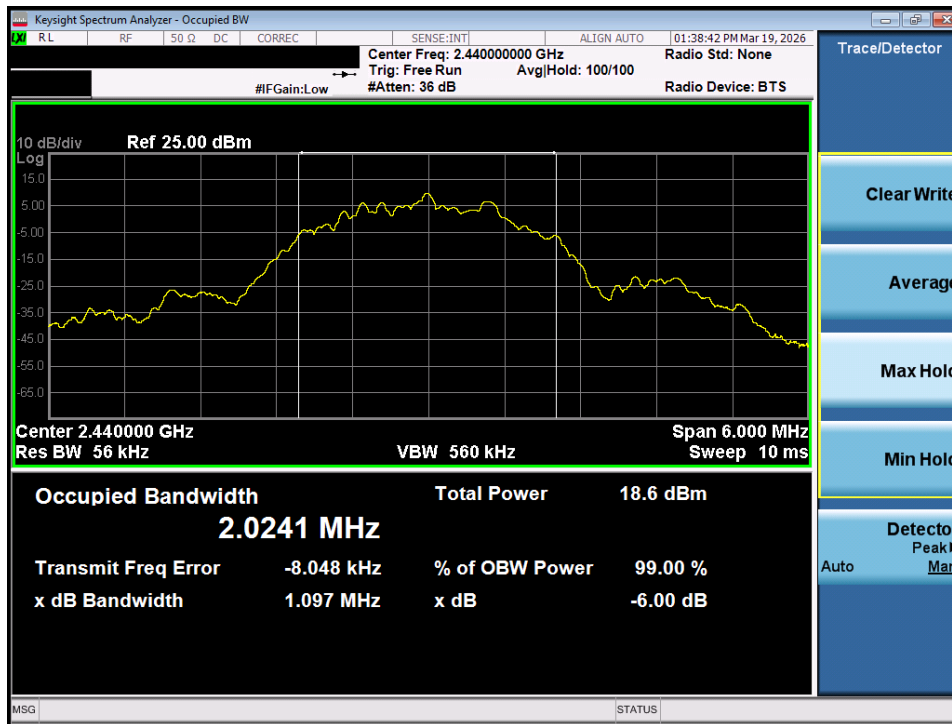
Plot 7-71. OBW Plot (Bluetooth (LE), 2Mbps – Ch. 17) – Dual ANT2
