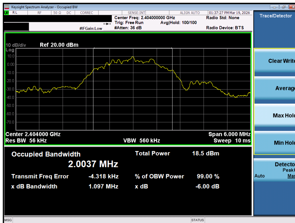
Plot 7-70. OBW Plot (Bluetooth (LE), 2Mbps – Ch. 0) – Dual ANT2
