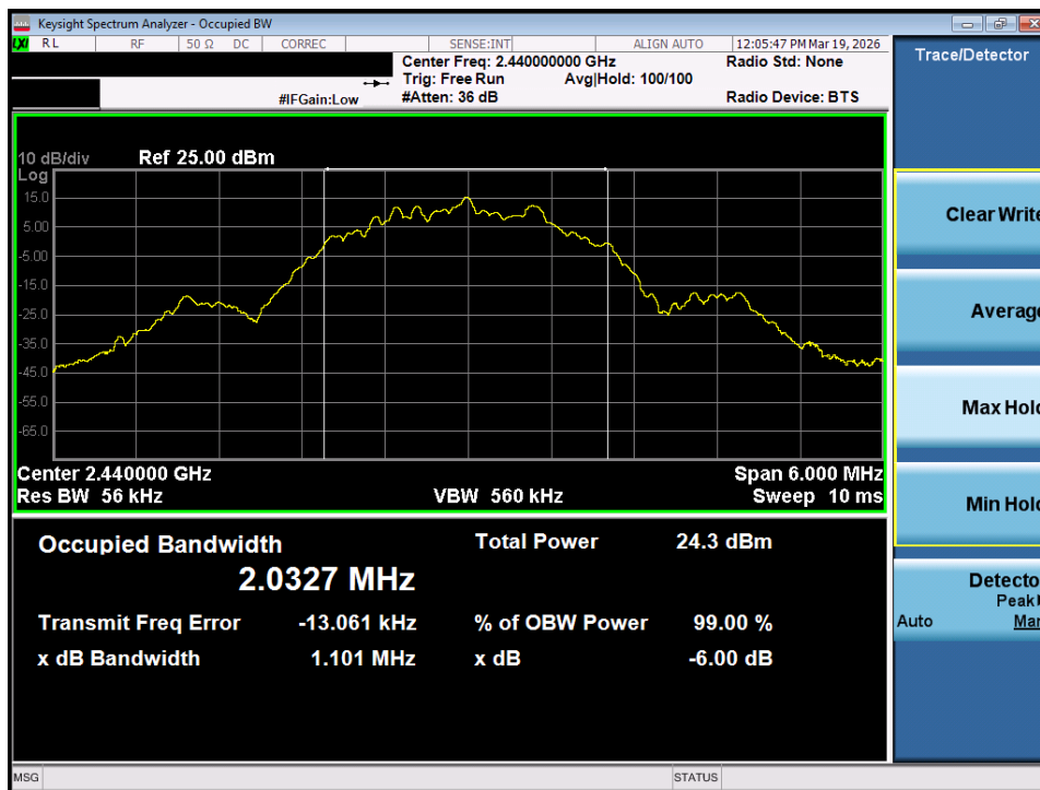
Plot 7-59. OBW Plot (Bluetooth (LE), 2Mbps – Ch. 17) – SISO ANT2
