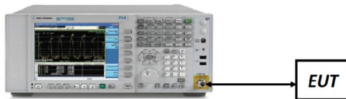
Figure 7-3. Test Instrument & Measurement Setup
