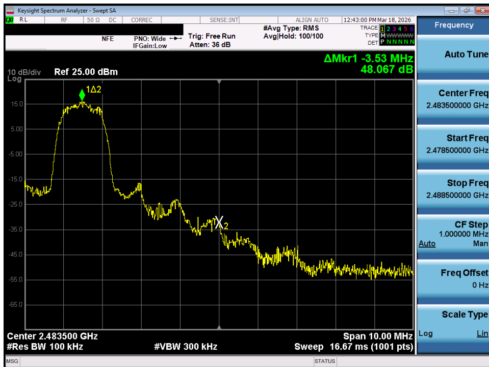
Plot 7-110. Band Edge Plot (Bluetooth with Hopping Disabled, 3 Mbps – Ch. 78) – SISO ANT 1
