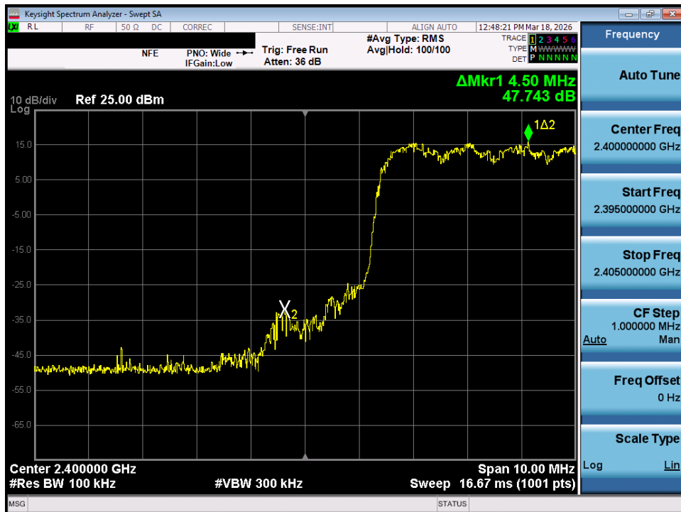
Plot 7-111. Band Edge Plot (Bluetooth with Hopping Enabled, 3 Mbps) – SISO ANT 1
