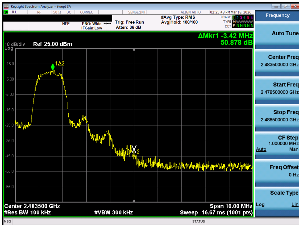
Plot 7-118. Band Edge Plot (Bluetooth with Hopping Disabled, 3 Mbps – Ch. 78) – MIMO ANT 1
