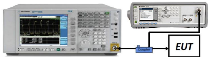
Figure 7-3. Test Instrument & Measurement Setup
