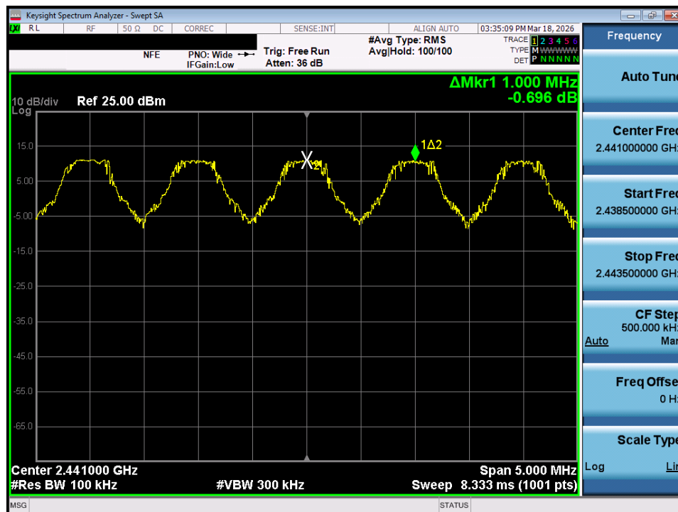
Plot 7-128. Channel Spacing Plot (Bluetooth) – MIMO Ant 2
