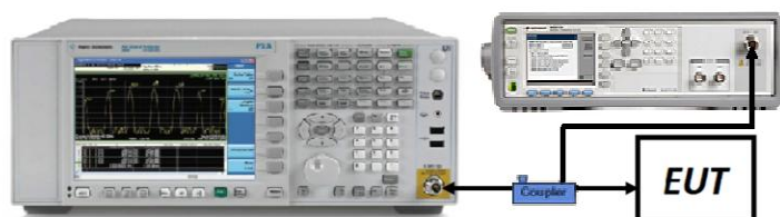
Figure 7-6. Test Instrument & Measurement Setup
