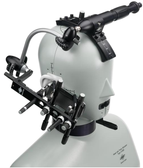
Figure 4-3 Head and Torso Simulator (with Handset Positioner)
