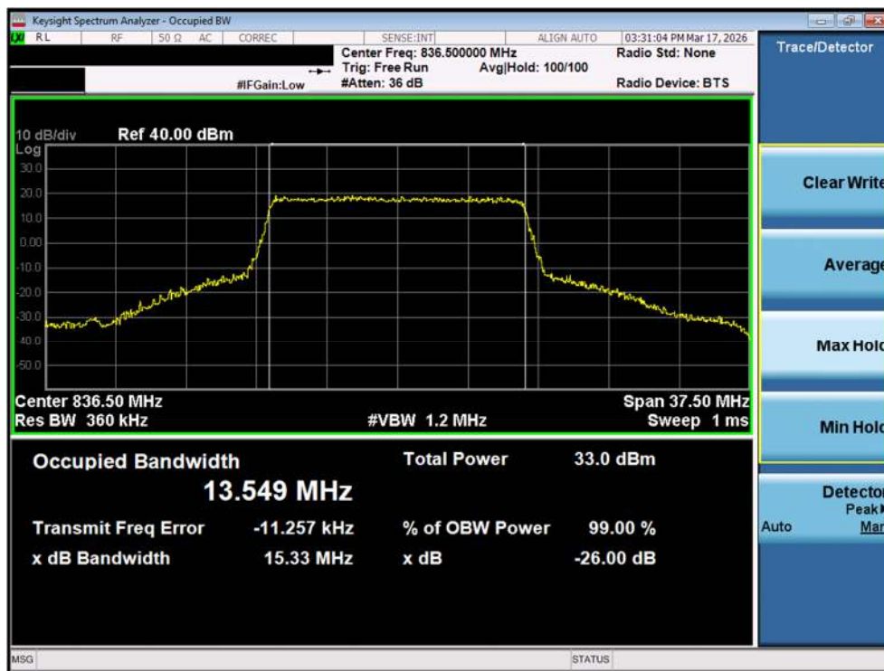
Plot 7-29. Occupied Bandwidth Plot (LTE Band 26 - 15MHz QPSK - Full RB – Ant2)
