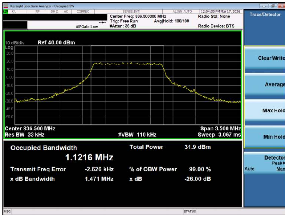
Plot 7-12. Occupied Bandwidth Plot (LTE Band 26/5 – 1.4MHz QPSK - Full RB – Ant1)
