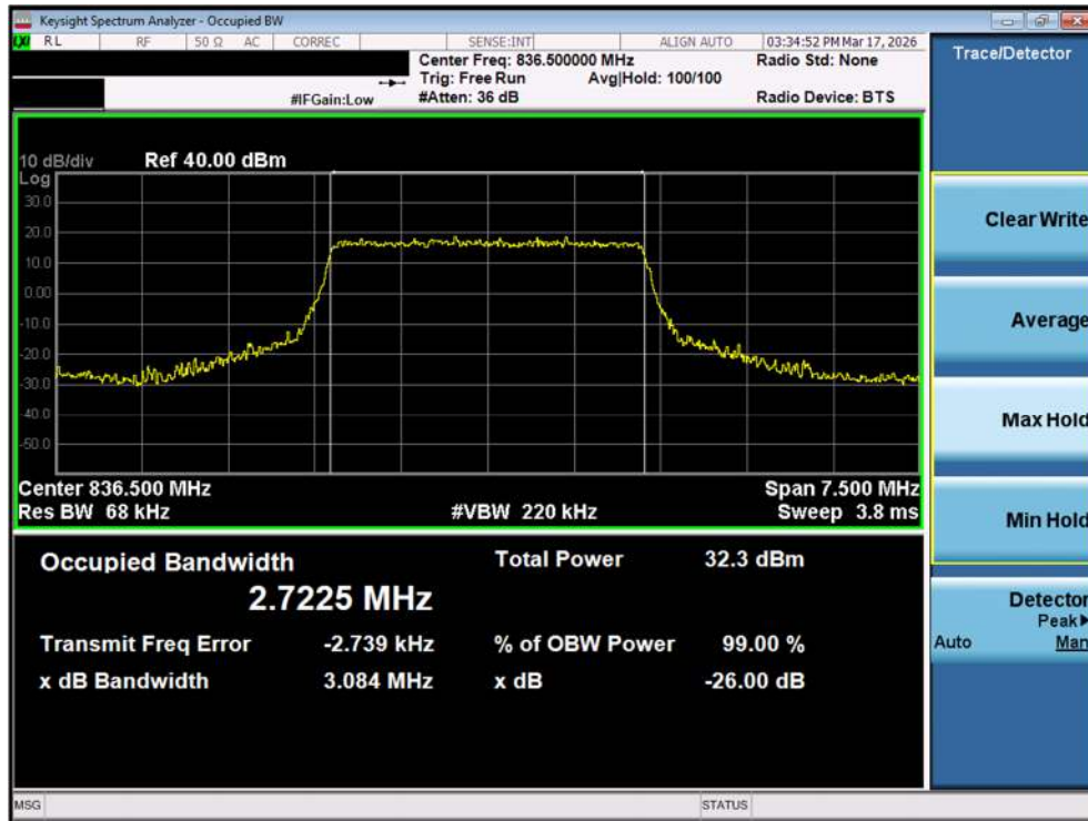
Plot 7-35. Occupied Bandwidth Plot (LTE Band 26/5 - 3MHz QPSK - Full RB – Ant2)
