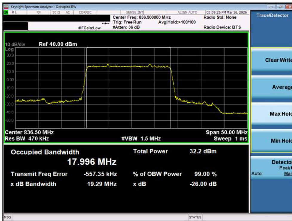
Plot 7-14. Occupied Bandwidth Plot (NR Band n26/5 - 20MHz \pi/2 BPSK - Full RB – Ant1)
