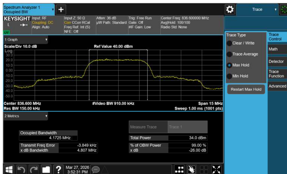
Plot 7-28. Occupied Bandwidth Plot (WCDMA 850 – Ant2)
