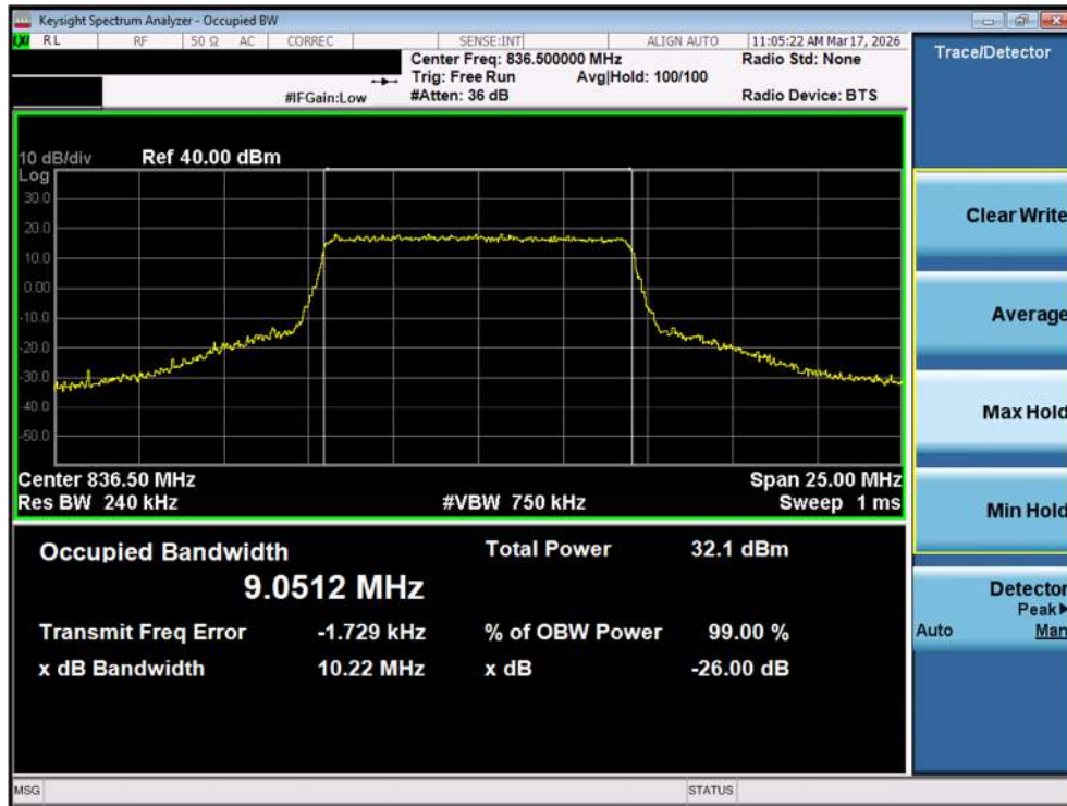
Plot 7-6. Occupied Bandwidth Plot (LTE Band 26/5 - 10MHz QPSK - Full RB – Ant1)
