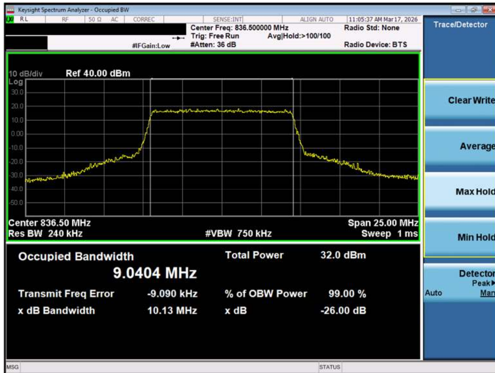
Plot 7-7. Occupied Bandwidth Plot (LTE Band 26/5 - 10MHz 16-QAM - Full RB – Ant1)
