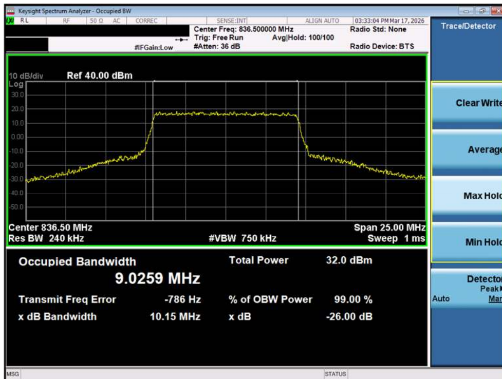
Plot 7-32. Occupied Bandwidth Plot (LTE Band 26/5 - 10MHz 16-QAM - Full RB – Ant2)
