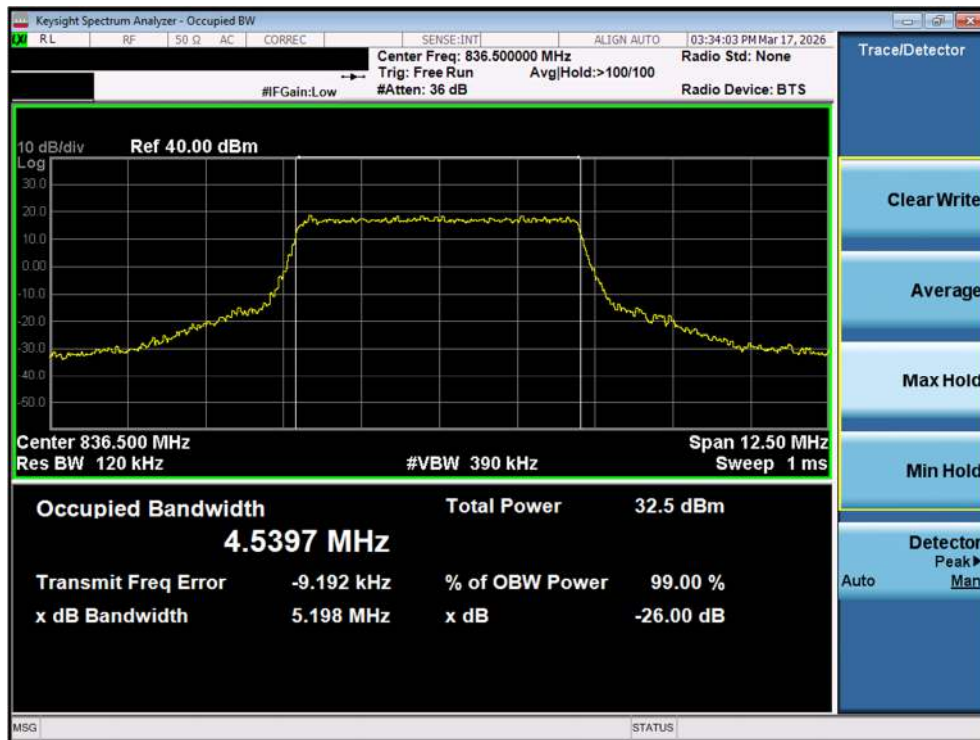
Plot 7-33. Occupied Bandwidth Plot (LTE Band 26/5 - 5MHz QPSK - Full RB – Ant2)
