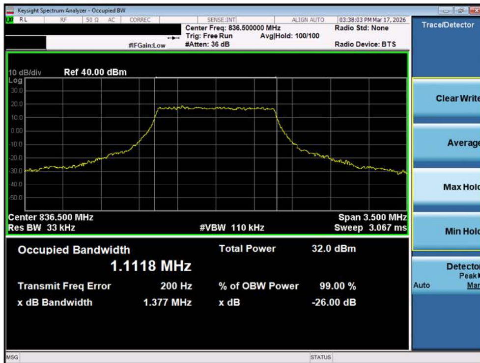
Plot 7-38. Occupied Bandwidth Plot (LTE Band 26/5 – 1.4MHz 16-QAM - Full RB - Ant2)
