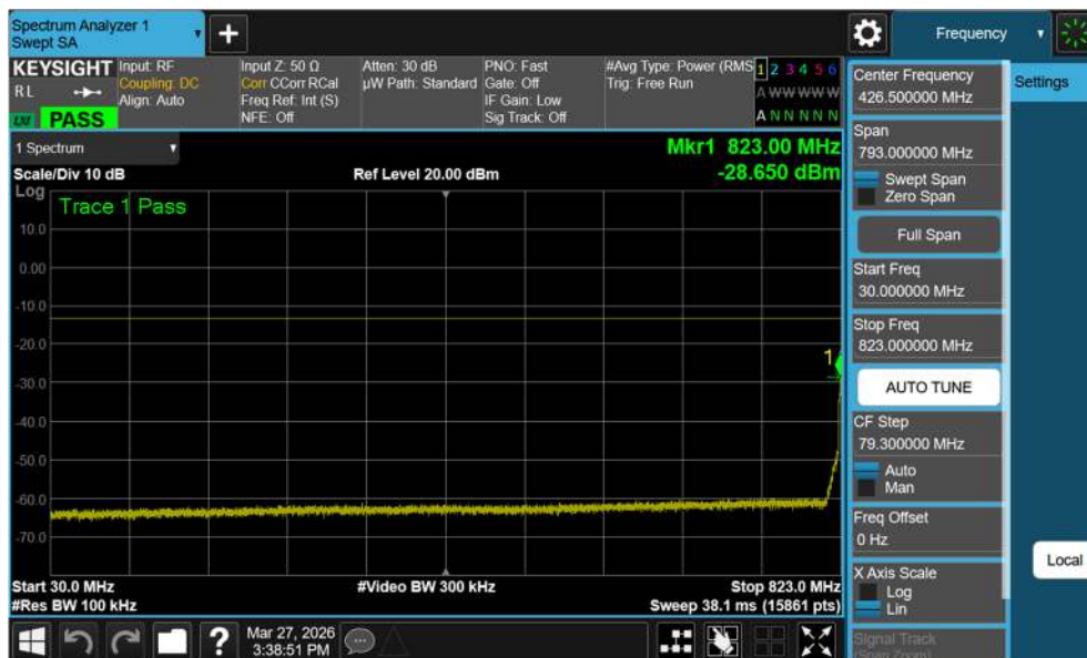
Plot 7-54. Conducted Spurious Plot (WCDMA – Low Channel – Ant1)
