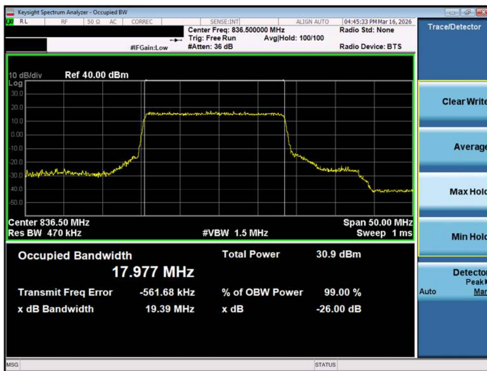
Plot 7-40. Occupied Bandwidth Plot (NR Band n26/5 - 20MHz QPSK - Full RB – Ant2)
