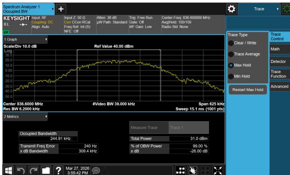
Plot 7-27. Occupied Bandwidth Plot (EDGE, Ch. 190 – Ant2)
