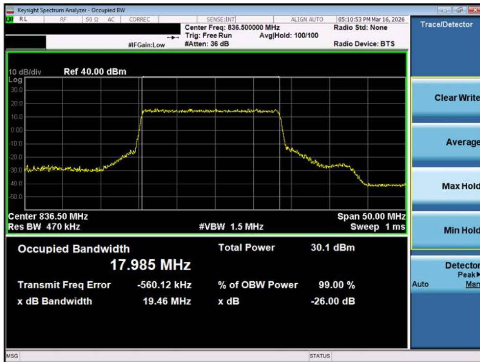
Plot 7-16. Occupied Bandwidth Plot (NR Band n26/5 - 20MHz 16-QAM - Full RB – Ant1)
