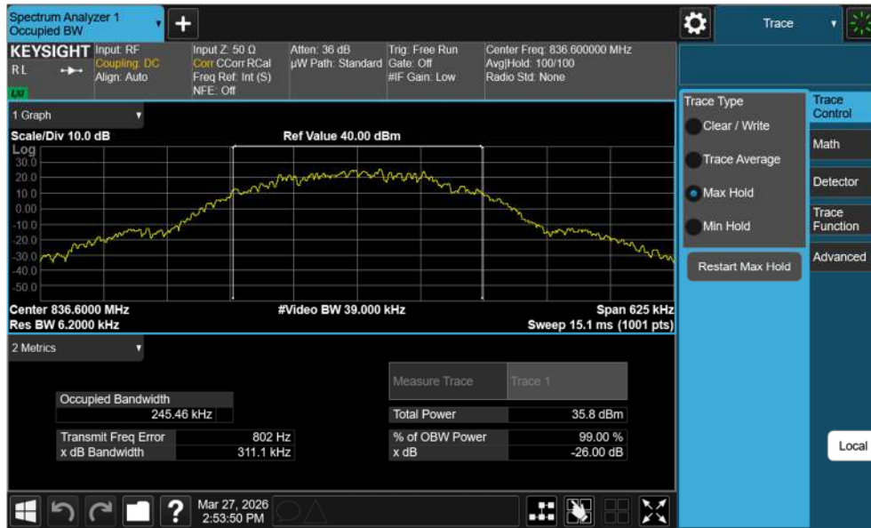
Plot 7-1. Occupied Bandwidth Plot (GPRS, Ch. 190 – Ant1)
