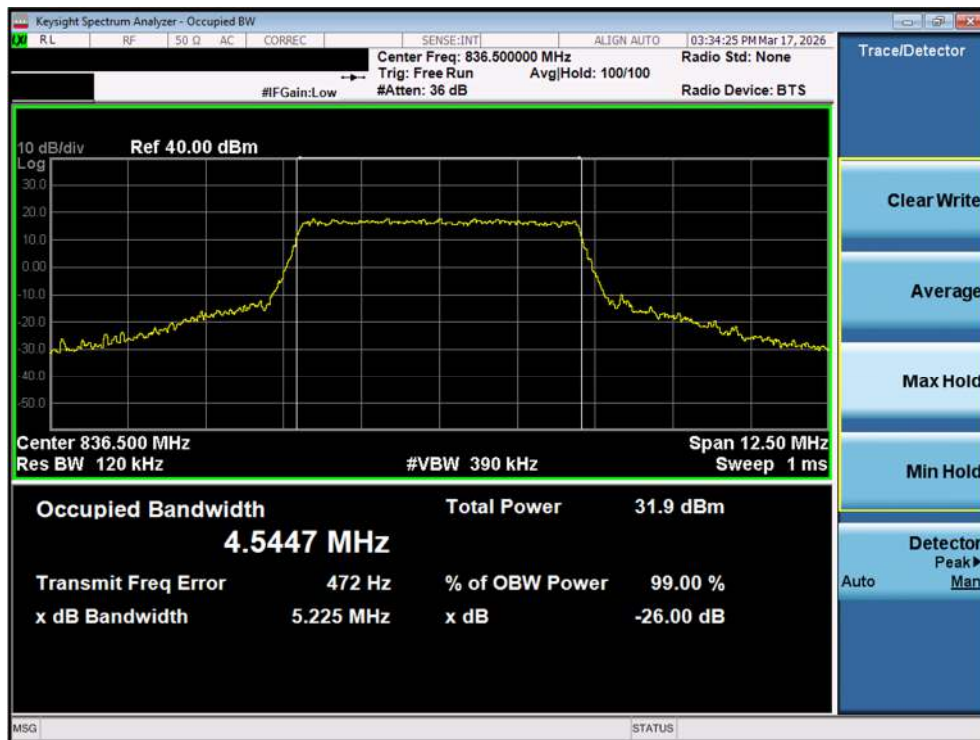
Plot 7-34. Occupied Bandwidth Plot (LTE Band 26/5 - 5MHz 16-QAM - Full RB – Ant2)
