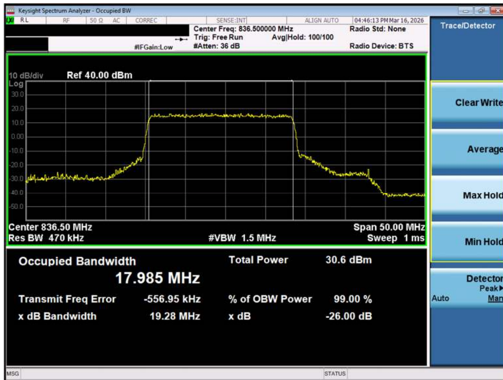
Plot 7-41. Occupied Bandwidth Plot (NR Band n26/5 - 20MHz 16-QAM - Full RB – Ant2)
