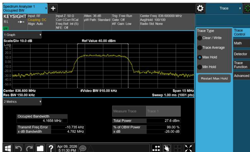
Plot 7-3. Occupied Bandwidth Plot (WCDMA 850 – Ant1)
