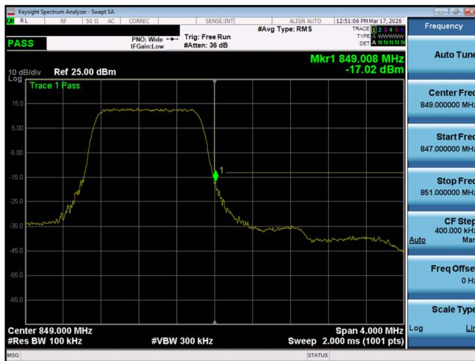
Plot 7-80. Upper Band Edge Plot (LTE Band 26/5 – 1.4MHz QPSK - Full RB – Ant1)
