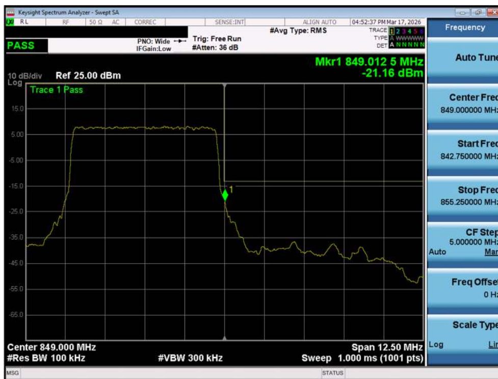
Plot 7-90. Upper Band Edge Plot (NR Band n26/5 – 5MHz - Full RB – Ant2)
