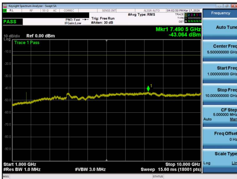
Plot 7-71. Conducted Spurious Plot (LTE Band 26/5 - 10MHz QPSK - 1 RB - High Channel – Ant2)
