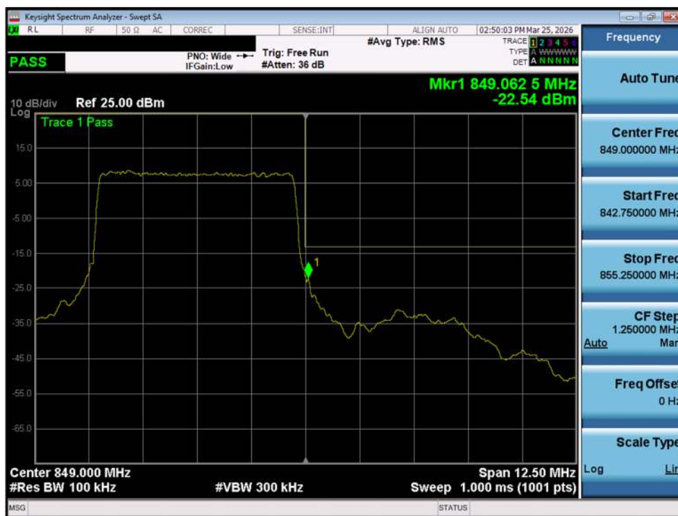
Plot 7-82. Upper Band Edge Plot (NR Band n26/5 – 5MHz - Full RB – Ant1)
