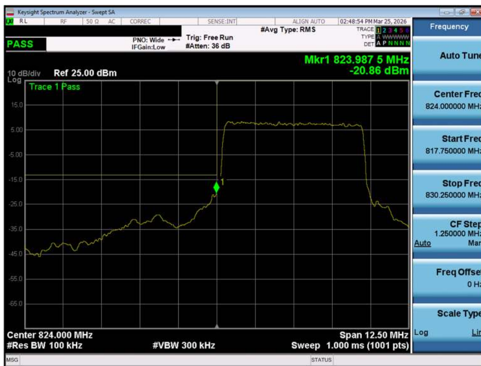
Plot 7-81. Lower Band Edge Plot (NR Band n26/5 – 5MHz - Full RB – Ant1)
