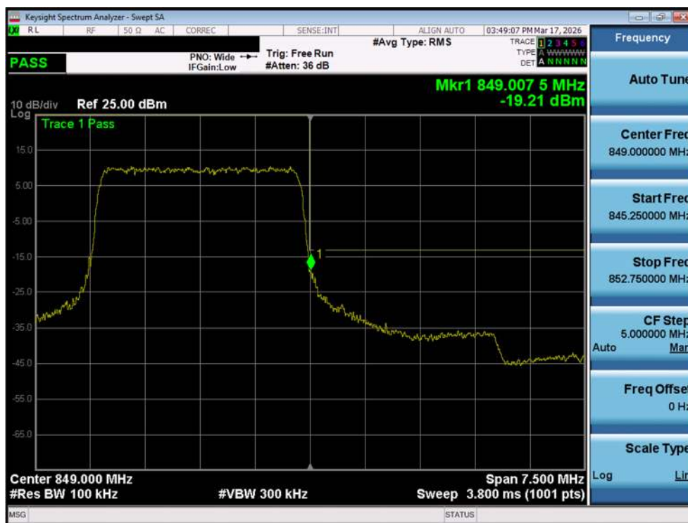
Plot 7-88. Upper Band Edge Plot (LTE Band 26/5 – 3MHz QPSK - Full RB – Ant2)
