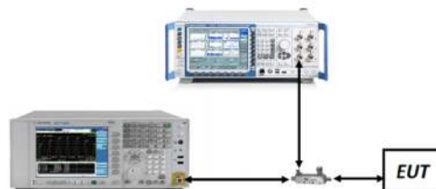
Figure 7-4. Test Instrument & Measurement Setup
