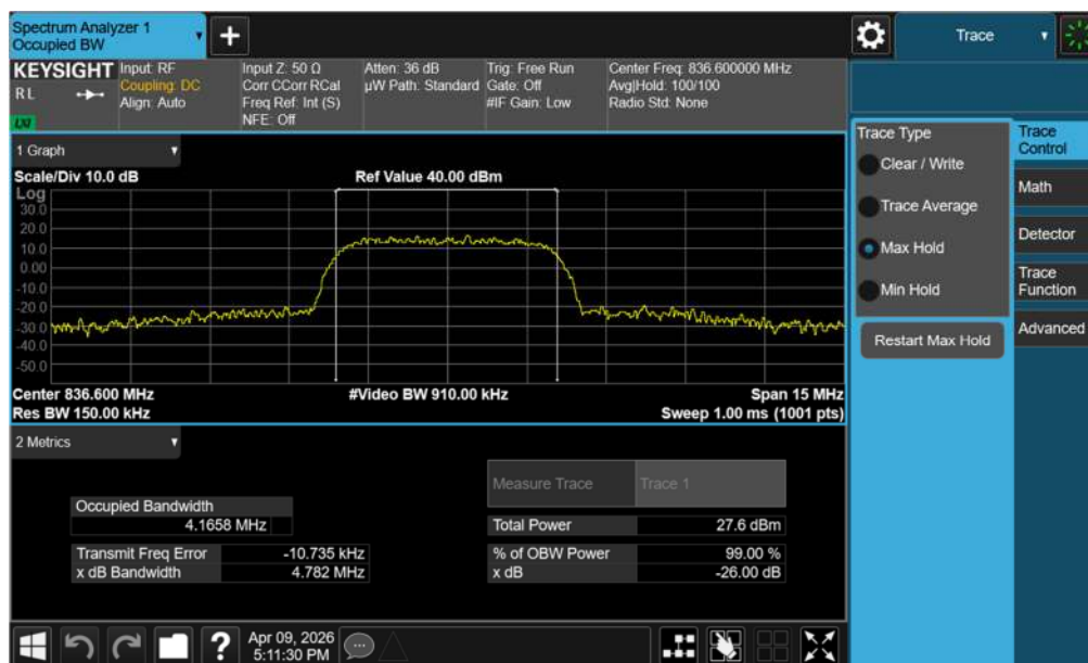
Plot 7-3. Occupied Bandwidth Plot (WCDMA, Ch. 9400 – Ant1)
