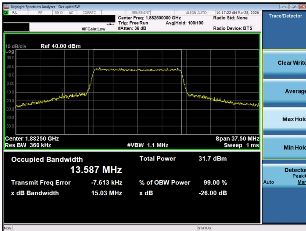
Plot 7-7. Occupied Bandwidth Plot (LTE Band 25/2 - 15MHz 16-QAM - Full RB - Ant1)
