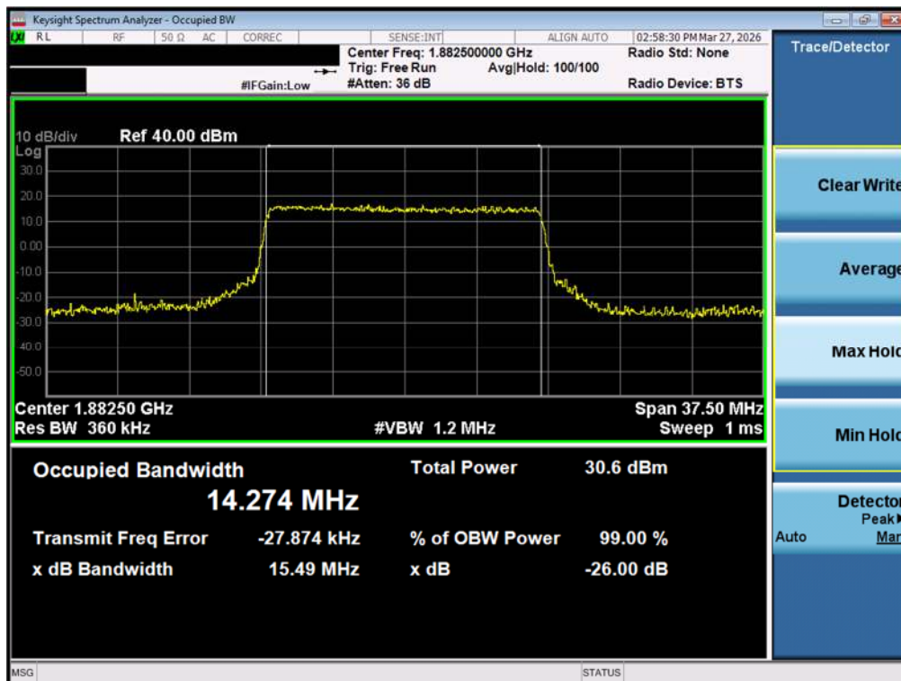
Plot 7-33. Occupied Bandwidth Plot (NR Band n25/2 - 15.0MHz CP-OFDM 16QAM - Full RB - ANT1)
