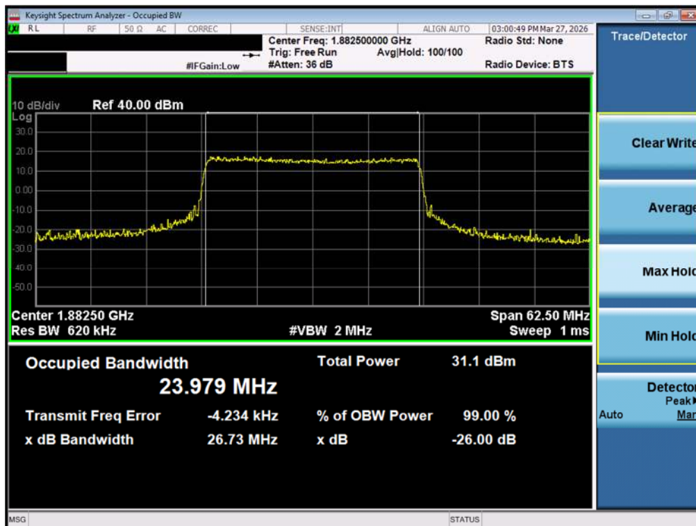
Plot 7-27. Occupied Bandwidth Plot (NR Band n25/2 - 25.0MHz CP-OFDM 16QAM - Full RB - ANT1)
