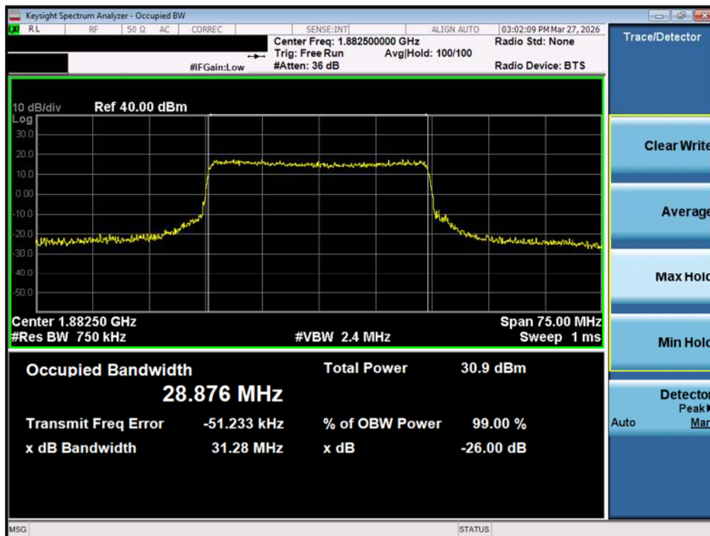
Plot 7-23. Occupied Bandwidth Plot (NR Band n25/2 - 30.0MHz CP-OFDM QPSK - Full RB - ANT1)
