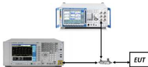
Figure 7-2. Test Instrument & Measurement Setup
