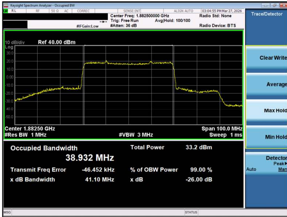
Plot 7-16. Occupied Bandwidth Plot (NR Band n25/2 - 40.0MHz DFT-s-OFDM BPSK - Full RB - ANT1)
