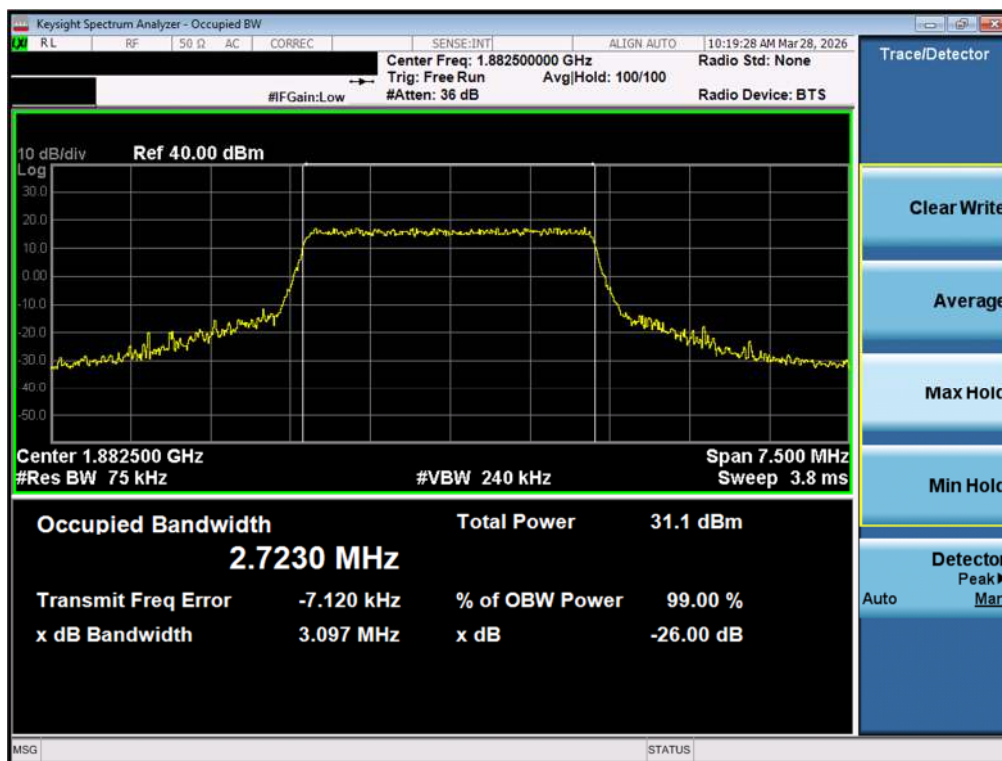
Plot 7-13. Occupied Bandwidth Plot (LTE Band 25/2 - 3MHz 16-QAM - Full RB - Ant1)
