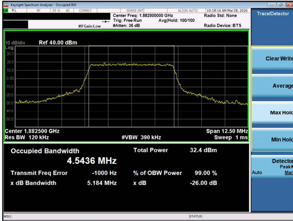
Plot 7-10. Occupied Bandwidth Plot (LTE Band 25/2 - 5MHz QPSK - Full RB - Ant1)
