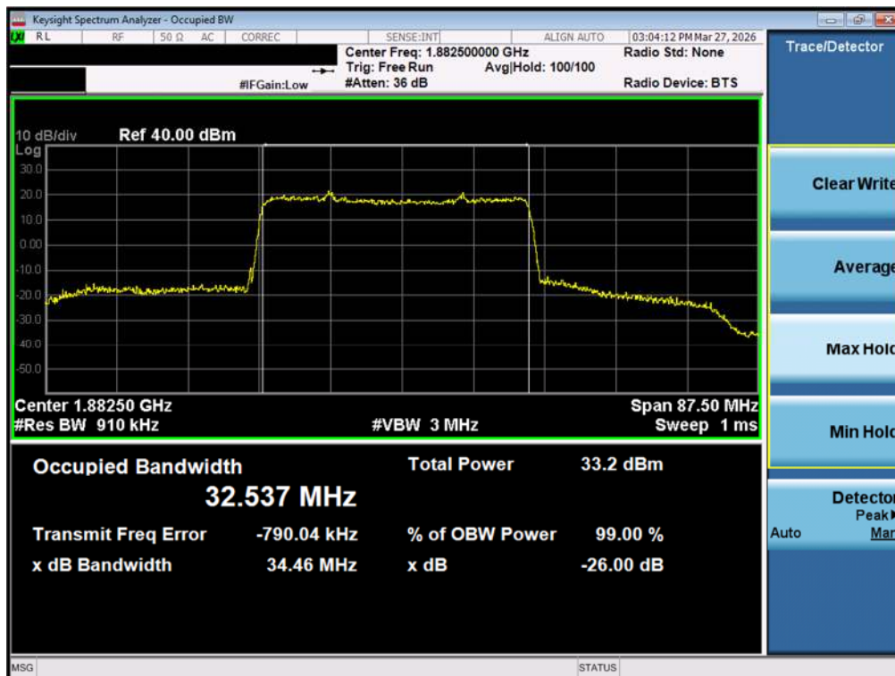
Plot 7-19. Occupied Bandwidth Plot (NR Band n25/2 - 35.0MHz DFT-s-OFDM BPSK - Full RB - ANT1)
