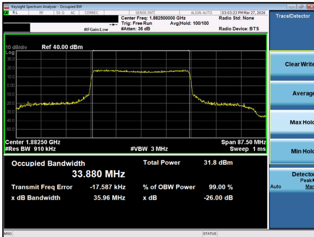
Plot 7-21. Occupied Bandwidth Plot (NR Band n25/2 - 35.0MHz CP-OFDM 16QAM - Full RB - ANT1)
