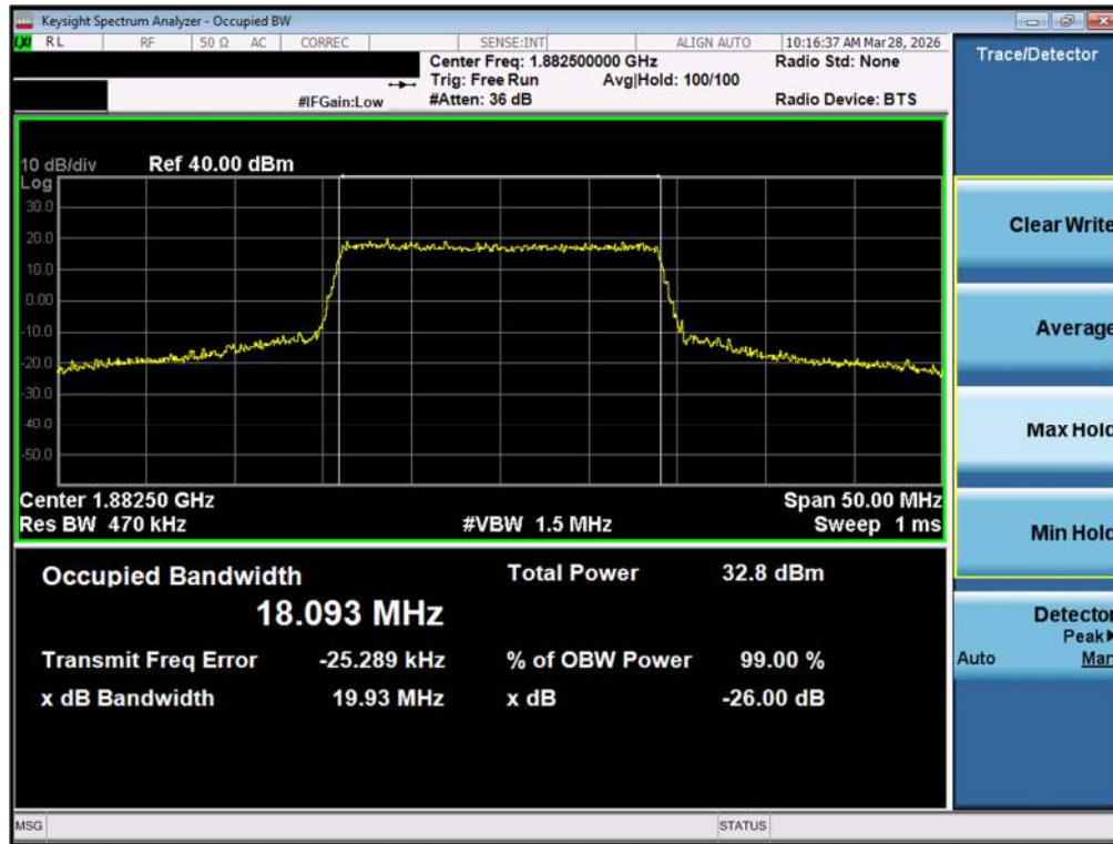
Plot 7-4. Occupied Bandwidth Plot (LTE Band 25/2 - 20MHz QPSK - Full RB - Ant1)
