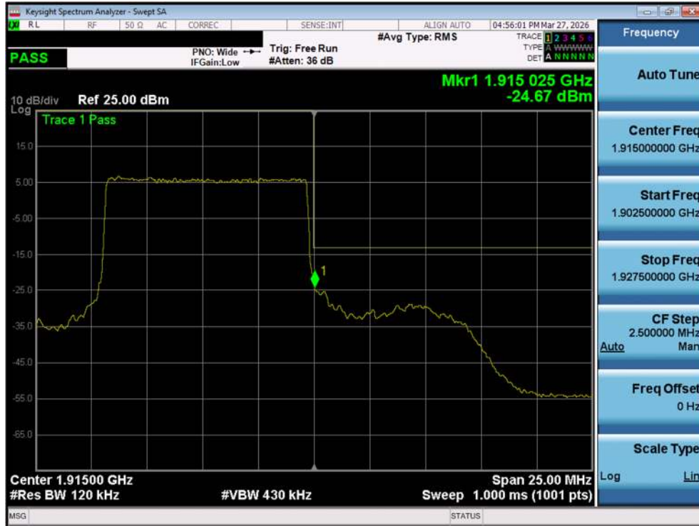
Plot 7-110. Upper Band Edge Plot (NR Band n25 - 10MHz QPSK – Full RB - Ant1)
