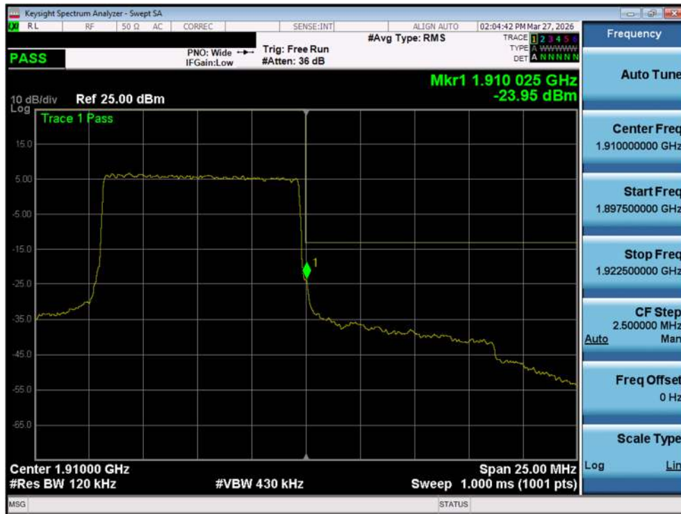
Plot 7-120. Upper Band Edge Plot (NR Band n2 - 10MHz QPSK – Full RB – Ant2)
