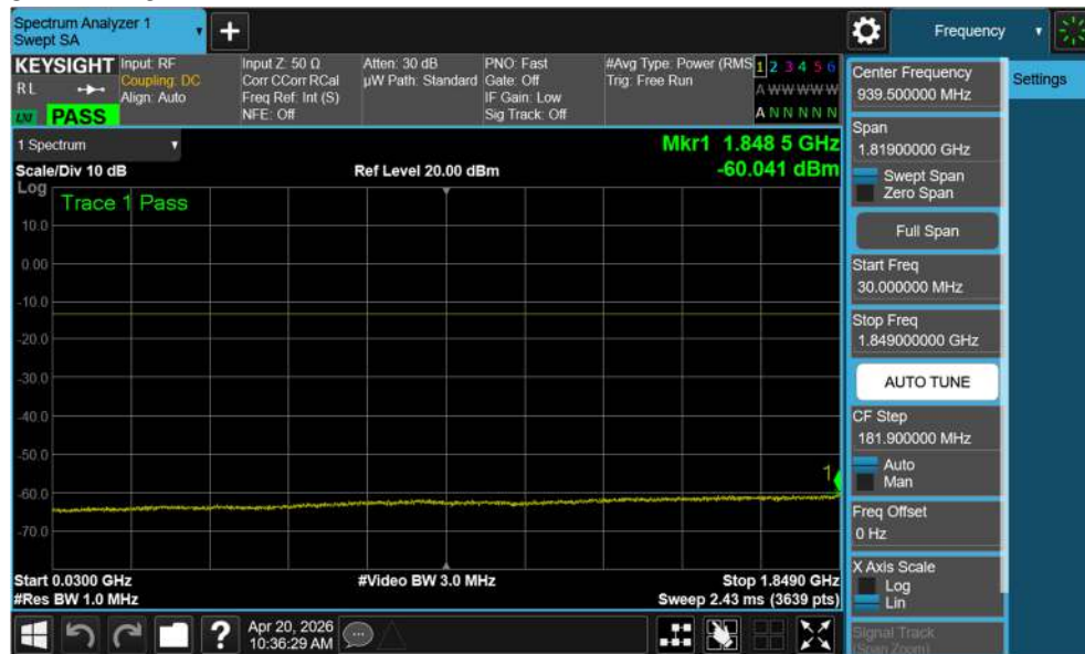
Plot 7-82. Conducted Spurious Plot (LTE Band 25/2 - 20MHz QPSK - 1RB - Low Channel - Ant1)
