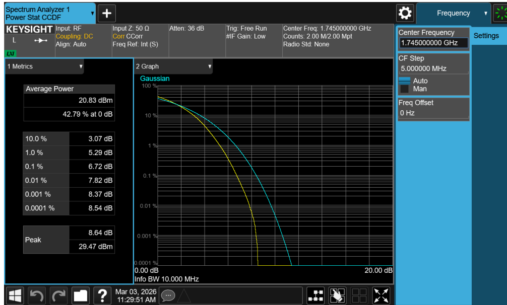
Plot 7-326. PAR Plot (LTE Band 66/4 - 10MHz 256-QAM - Full RB - ANT2)
