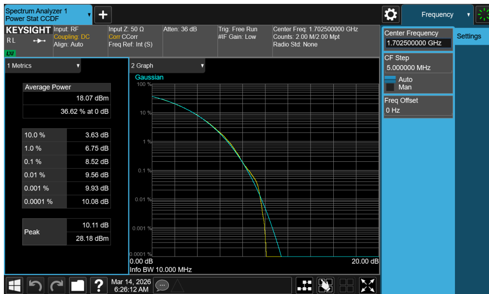
Plot 7-313. PAR Plot (NR Band n70 - 10.0MHz CP-OFDM 256-QAM - Full RB - ANT1)
