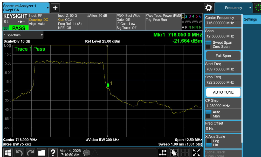
Plot 7-296. Upper Band Edge Plot (NR Band n12 – 5.0MHz - Full RB - ANT2)
