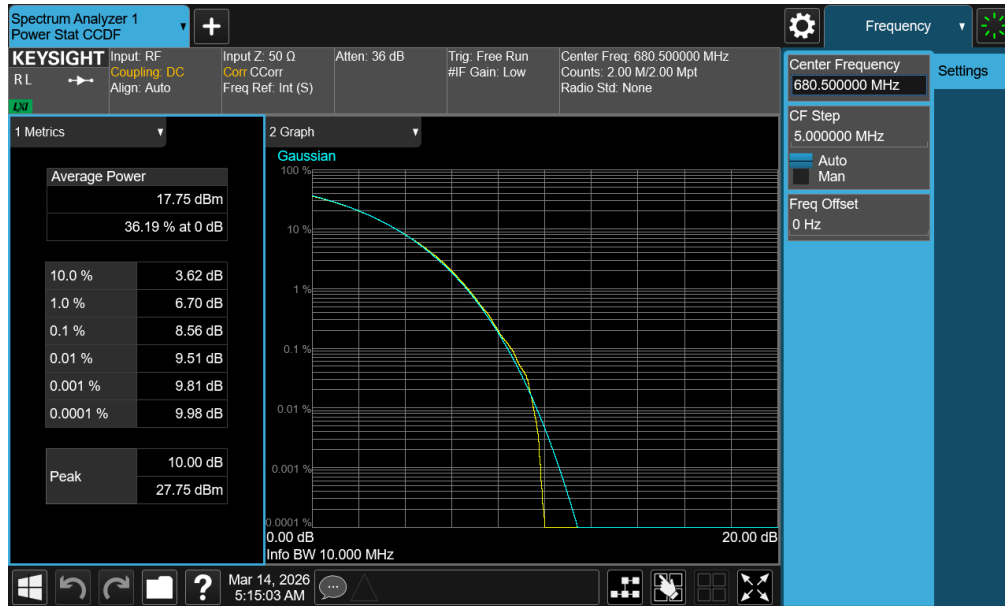
Plot 7-354. PAR Plot (NR Band n71 - 10.0MHz CP-OFDM 256-QAM - Full RB - ANT1)
