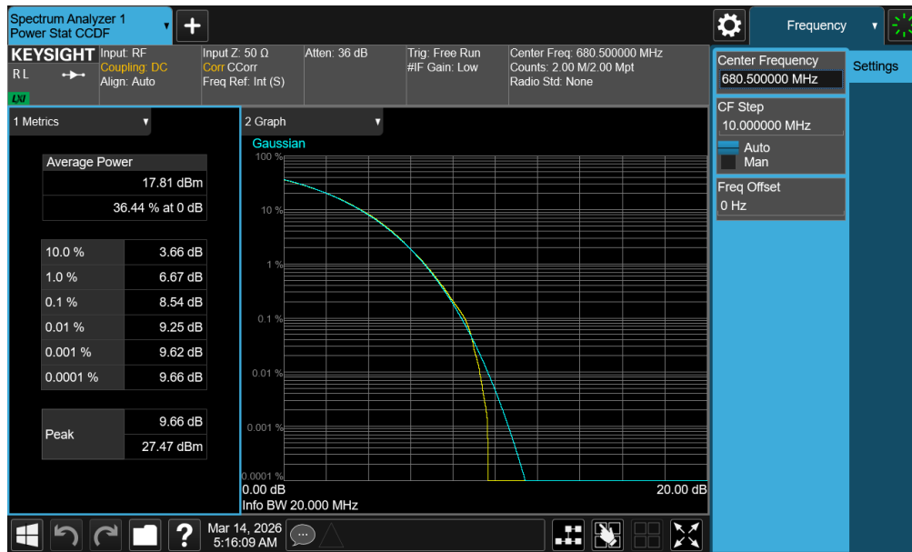
Plot 7-352. PAR Plot (NR Band n71 - 20.0MHz CP-OFDM 256-QAM - Full RB - ANT1)
