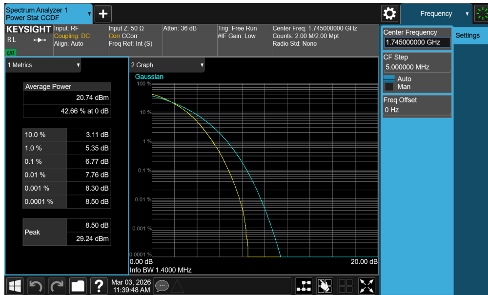
Plot 7-329. PAR Plot (LTE Band 66/4 - 1.4MHz 256-QAM - Full RB - ANT2)
