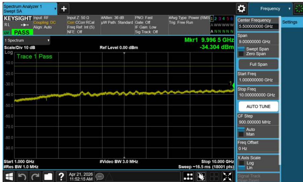
Plot 7-94. Conducted Spurious Plot (NR Band 26 - 20MHz QPSK - 1 RB - Mid Channel – Ant1)
