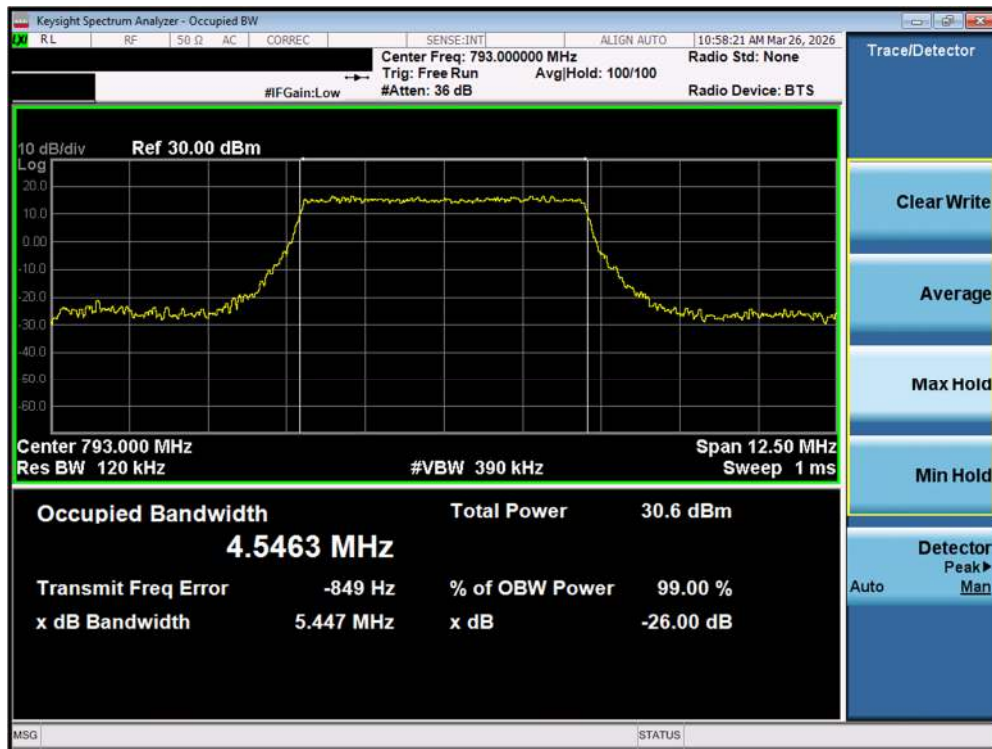
Plot 7-66. Occupied Bandwidth Plot (NR Band n14 - 5MHz QPSK - Full RB)
