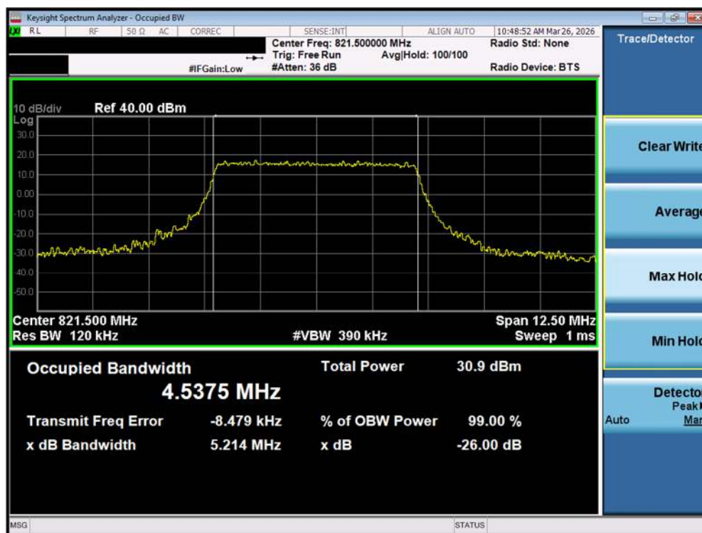
Plot 7-82. Occupied Bandwidth Plot (NR Band n26 – 5MHz 16-QAM High Channel - Full RB)
