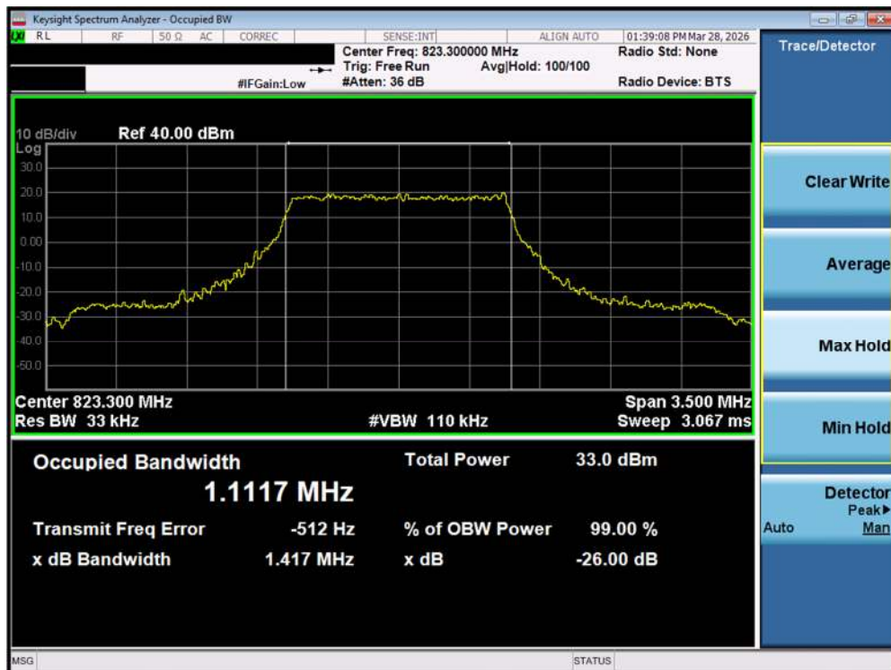
Plot 7-59. Occupied Bandwidth Plot (LTE Band 26 – 1.4MHz QPSK High Channel - Full RB)
