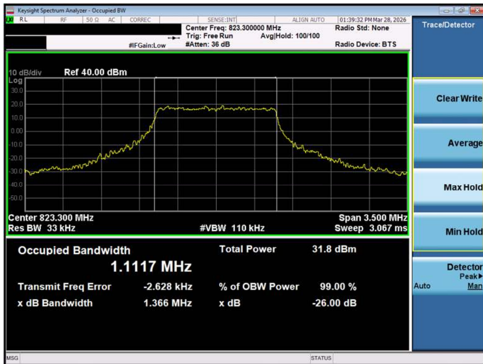
Plot 7-61. Occupied Bandwidth Plot (LTE Band 26 – 1.4MHz 16-QAM High Channel - Full RB)
