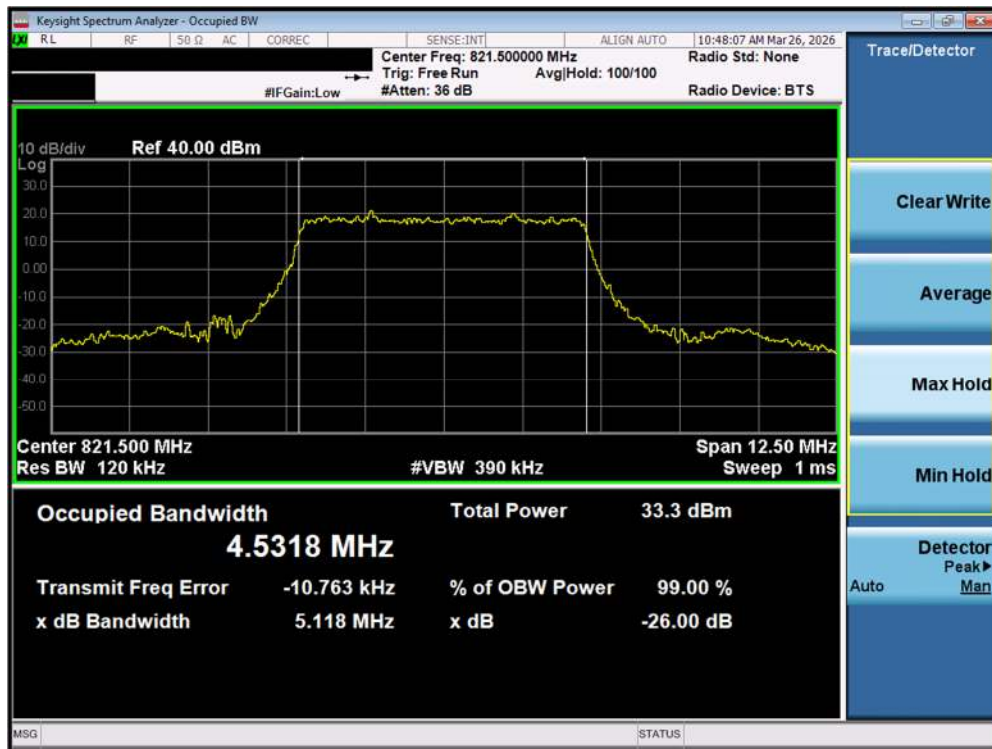
Plot 7-78. Occupied Bandwidth Plot (NR Band n26 – 5MHz \pi/2 BPSK High Channel - Full RB)
