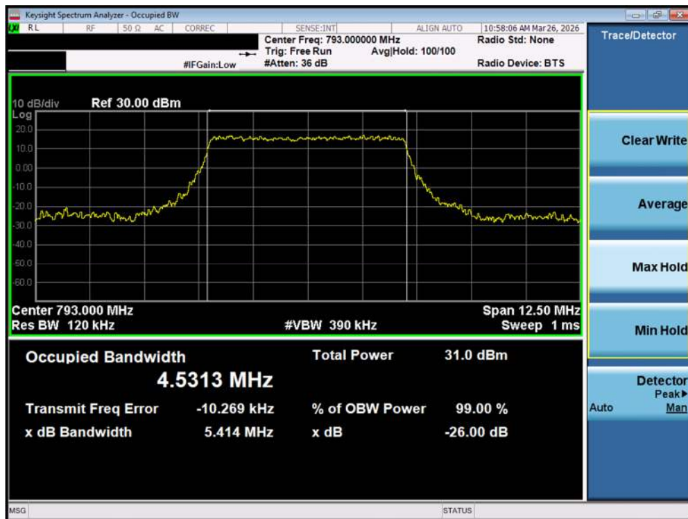
Plot 7-67. Occupied Bandwidth Plot (NR Band n14 - 5MHz 16-QAM - Full RB)
