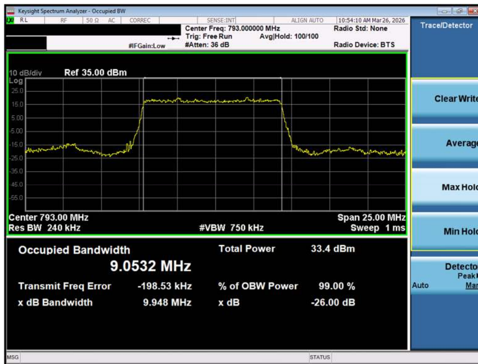
Plot 7-62. Occupied Bandwidth Plot (NR Band n14 - 10MHz \pi/2 BPSK - Full RB)
