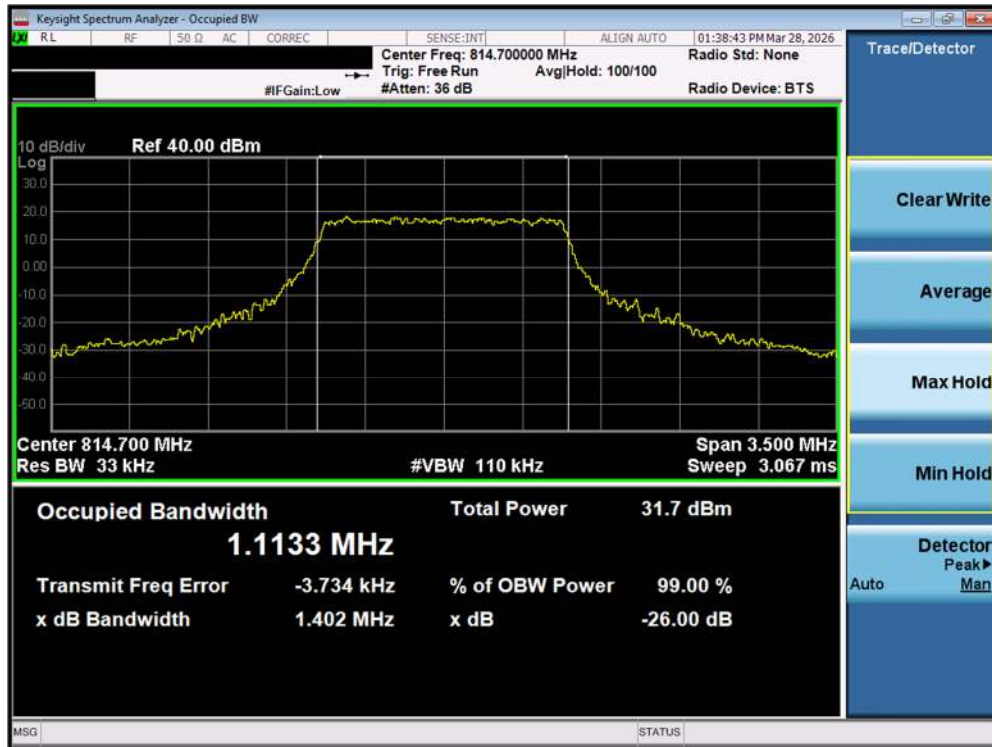
Plot 7-60. Occupied Bandwidth Plot (LTE Band 26 – 1.4MHz 16-QAM Low Channel - Full RB)
