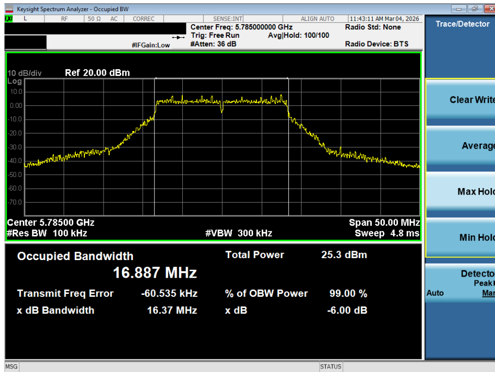
Plot 7-42. 6dB Bandwidth Plot MIMO ANT2 (802.11a (UNII Band 3) – Ch. 157)
