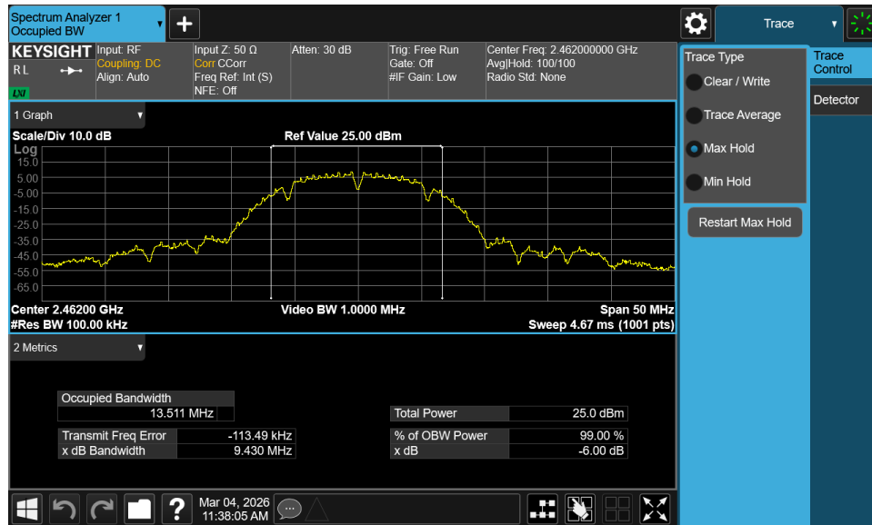
Plot 7-15. 6dB Bandwidth Plot MIMO ANT2 (802.11b – Ch. 11)
