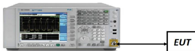
Figure 7-1. Test Instrument & Measurement Setup
