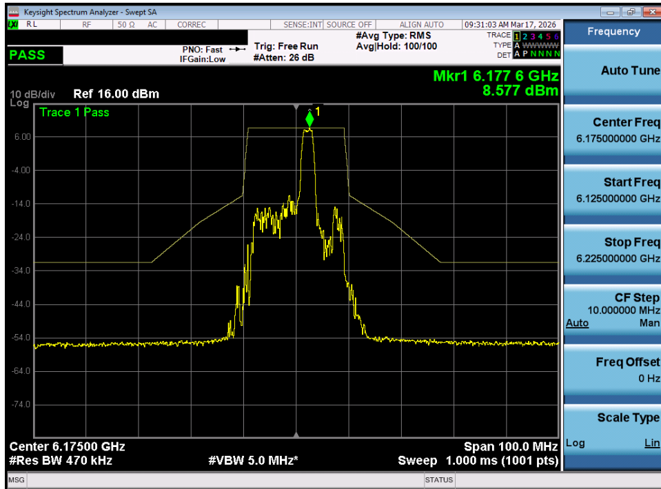
Plot 7-102. In Band Emissions Plot MIMO ANT1 (20MHz 802.11ax/be (26 Tones) (UNII Band 5) – Ch. 45) - SP
