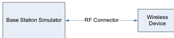
Figure 9-2 Power Measurement Setup
