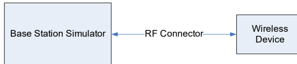
Figure 9-3 Power Measurement Setup
