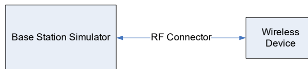
Figure 9-3 Power Measurement Setup
