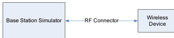
Figure 9-2 Power Measurement Setup
