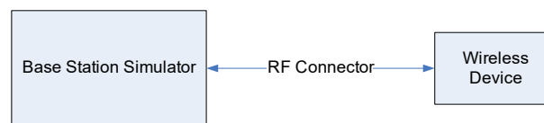
Figure 9-3 Power Measurement Setup
