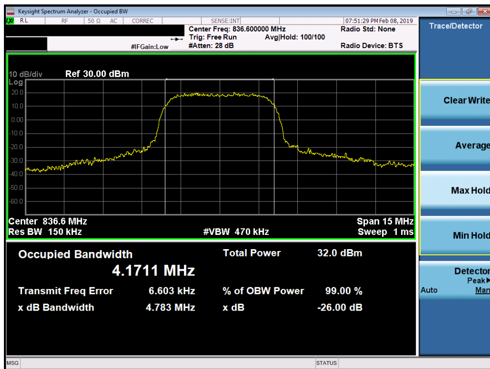
Plot 7-5. Occupied Bandwidth Plot (Cellular WCDMA Mode)
