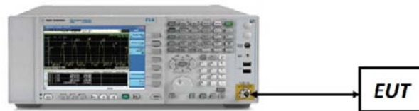
Figure 7-1. Test Instrument & Measurement Setup
