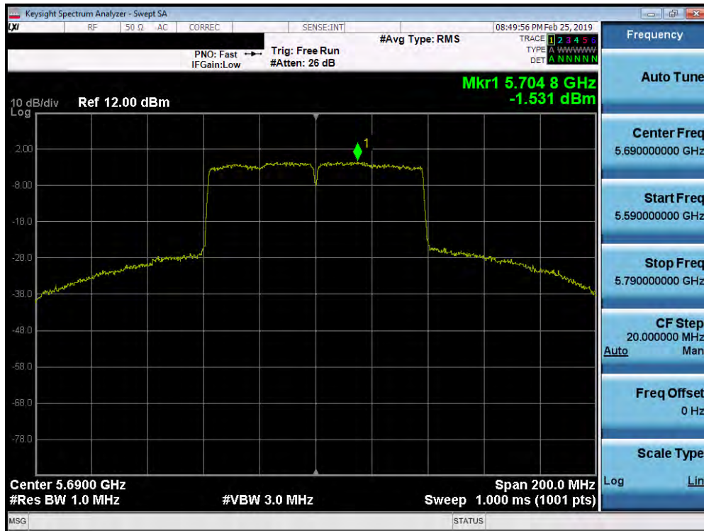
Plot 7-180. Power Spectral Density Plot SISO ANT1 (80MHz BW 802.11ac (UNII Band 2C) – Ch. 138)
