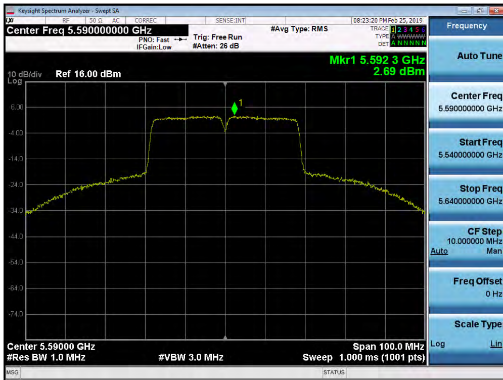
Plot 7-173. Power Spectral Density Plot SISO ANT1 (40MHz BW 802.11n (UNII Band 2C) – Ch. 118)
