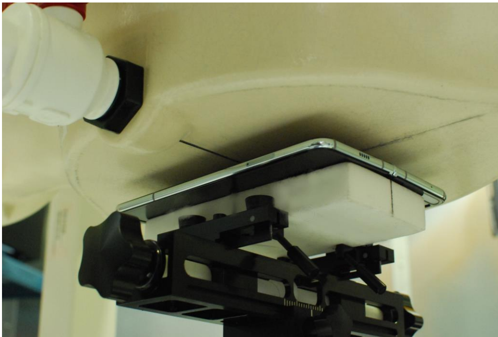
SAR Test Setup Photo 20 – Open Configuration (UMPC) Back Side at 12 mm
