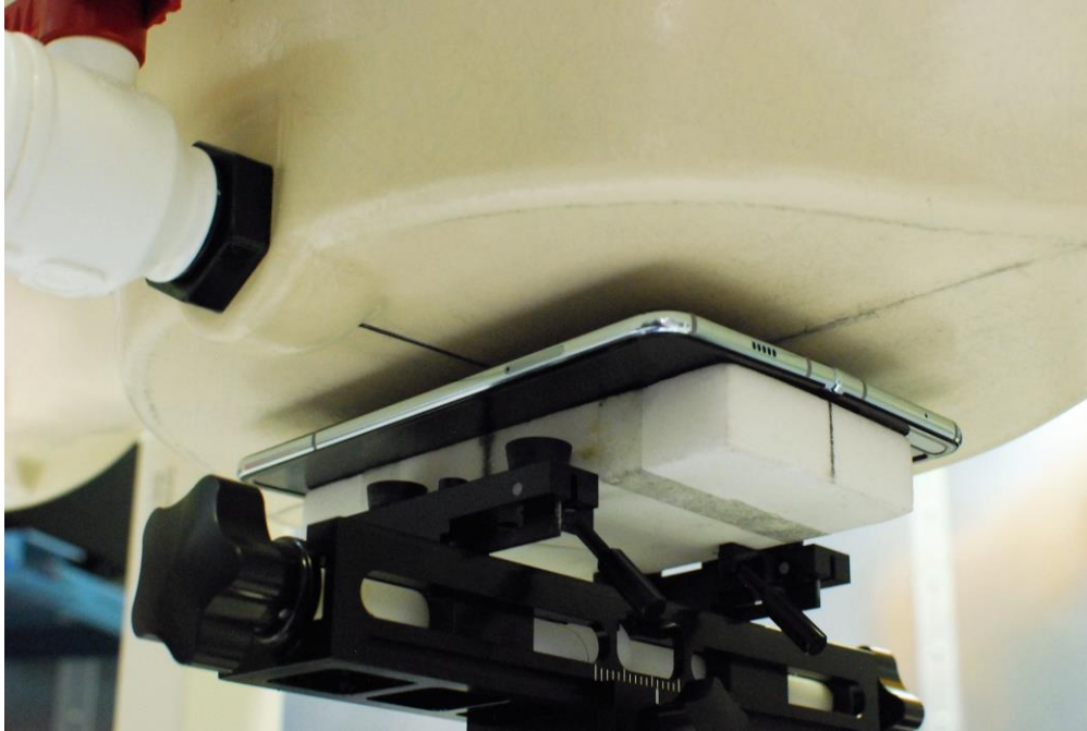
SAR Test Setup Photo 21 – Open Configuration (UMPC) Back Side at 10 mm
