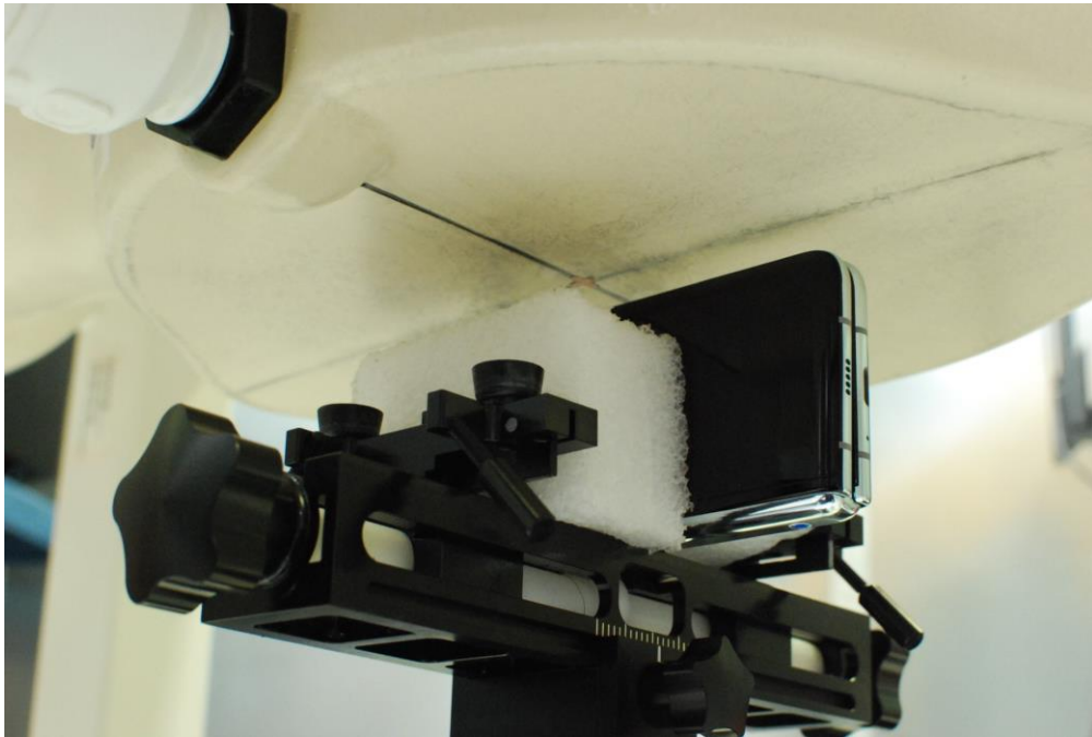
SAR Test Setup Photo 16 – Closed Configuration (Handset) Right Side at 10 mm
