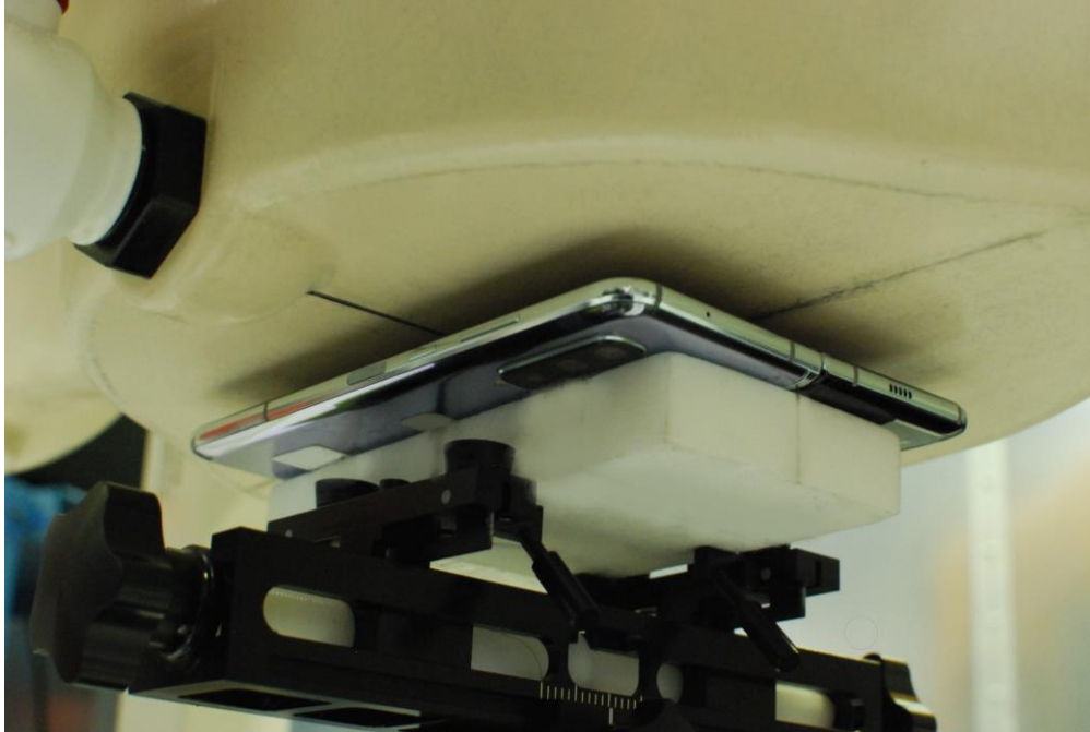
SAR Test Setup Photo 23 – Open Configuration (UMPC) Front Side at 11 mm
