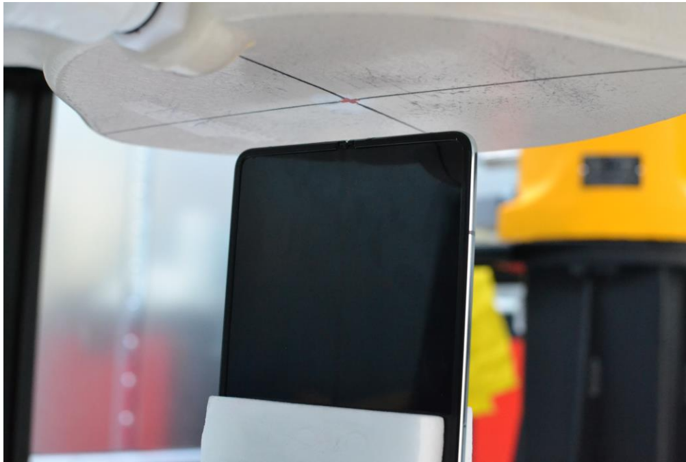
SAR Test Setup Photo 28 – Open Configuration (UMPC) Bottom Side at 16 mm
