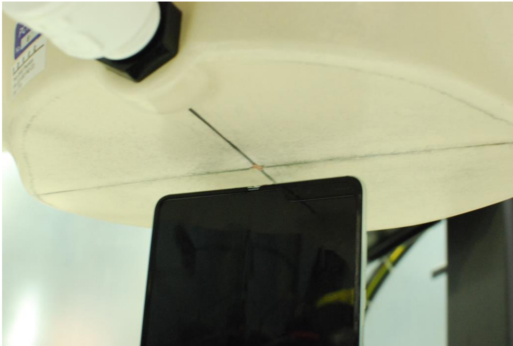
SAR Test Setup Photo 26 – Open Configuration (UMPC) Top Side at 10 mm
