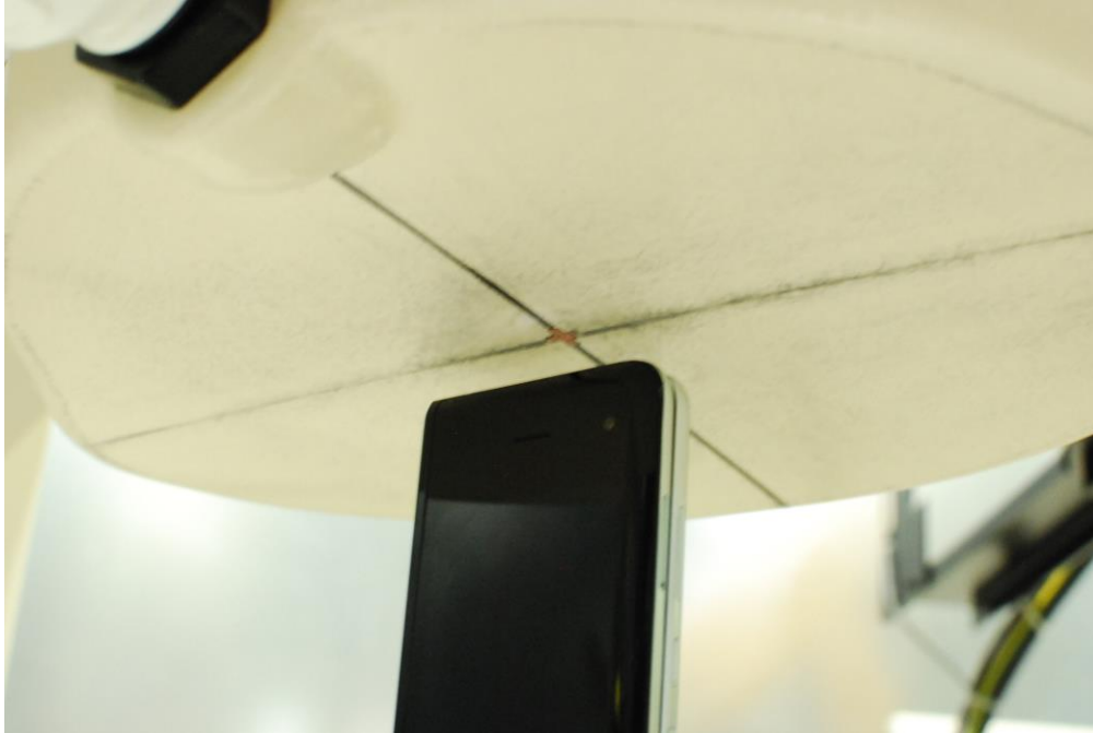
SAR Test Setup Photo 11 – Closed Configuration (Handset) Top Side at 10 mm
