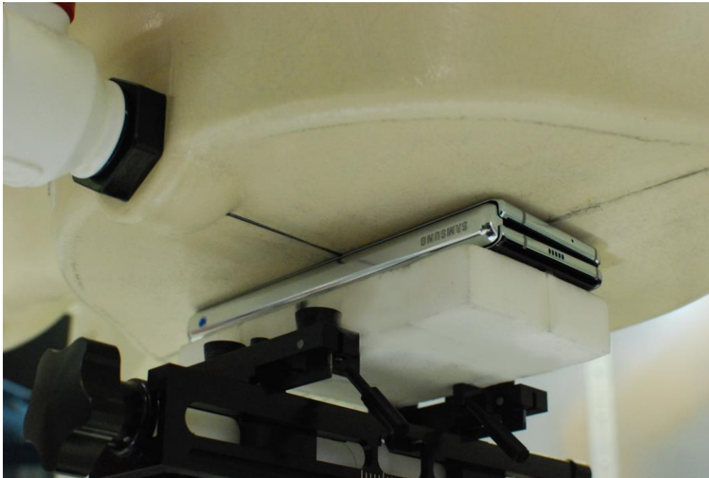
SAR Test Setup Photo 8 – Closed Configuration (Handset) Back Side at 0 mm
