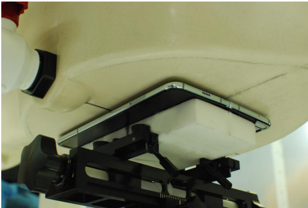
SAR Test Setup Photo 22 – Open Configuration (UMPC) Back Side at 0 mm
