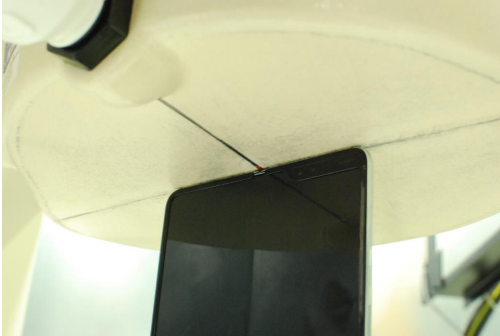
SAR Test Setup Photo 27 – Open Configuration (UMPC) Top Side at 0 mm
