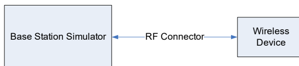
Figure 9-4 Power Measurement Setup
