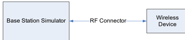
Figure 9-1 Power Measurement Setup
