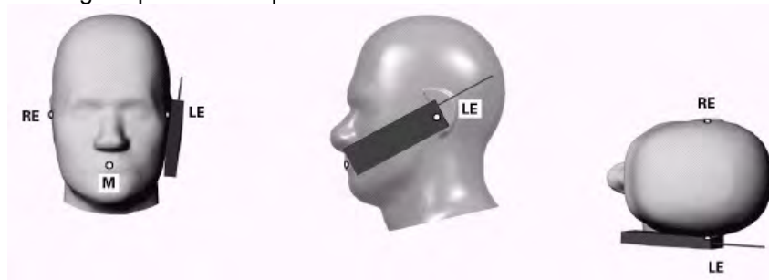
Figure 6-1 Front, Side and Top View of Cheek Position
