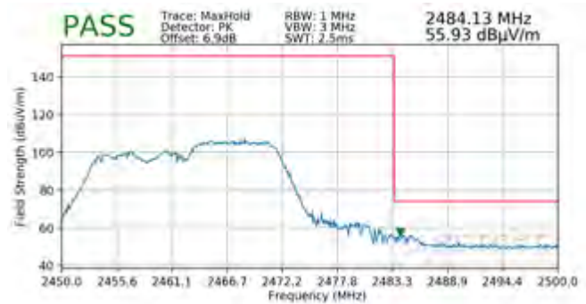
Plot 7-148. Radiated Restricted Upper Band Edge Measurement MIMO (Peak – 106 Tones)
