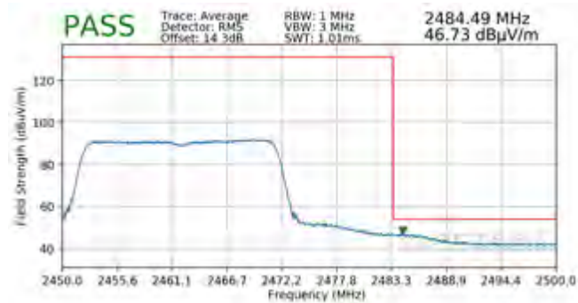
Plot 7-165. Radiated Restricted Band Edge Measurement MIMO with WCP (Average – 242 Tones)
