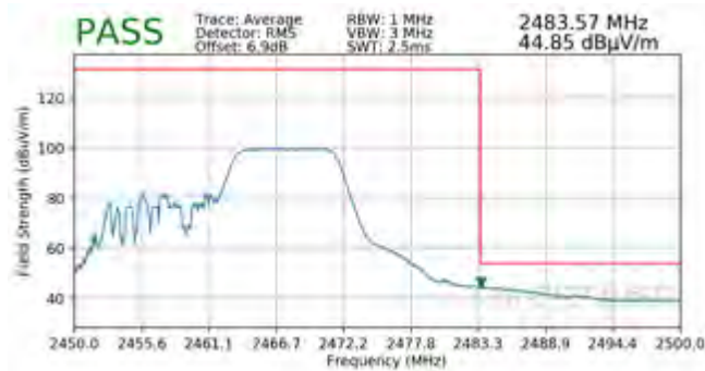
Plot 7-95. Radiated Restricted Upper Band Edge Measurement SISO ANT1 (Average – 106 Tones)
