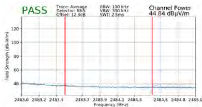
Plot 7-111. Radiated Restricted Upper Band Edge Measurement SISO ANT1 (Average – 242 Tones)
