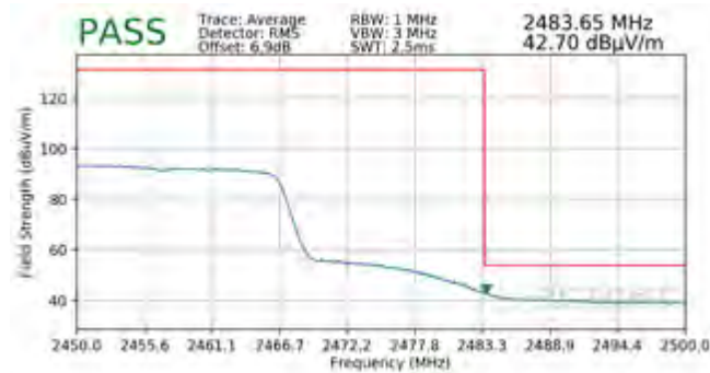
Plot 7-157. Radiated Restricted Upper Band Edge Measurement MIMO (Average – 242 Tones)
