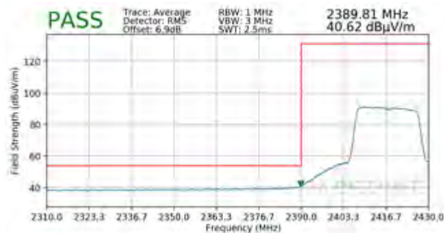
Plot 7-129. Radiated Restricted Lower Band Edge Measurement SISO ANT2 (Average – 242 Tones)
