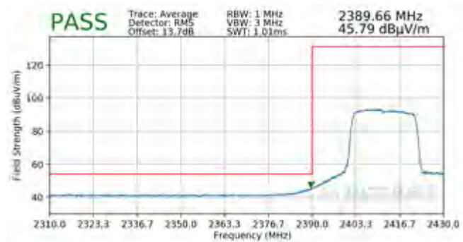
Plot 7-113. Radiated Restricted Band Edge Measurement SISO ANT1 with WCP (Average – 242 Tones)
