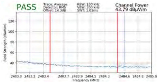
Plot 7-151. Radiated Restricted Upper Band Edge Measurement MIMO (Average – 26 Tones)
