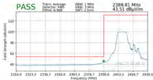
Plot 7-89. Radiated Restricted Lower Band Edge Measurement SISO ANT1 (Average – 106 Tones)
