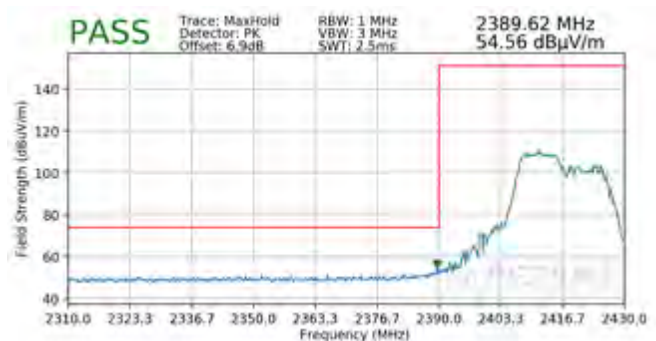
Plot 7-92. Radiated Restricted Lower Band Edge Measurement SISO ANT1 (Peak – 106 Tones)
