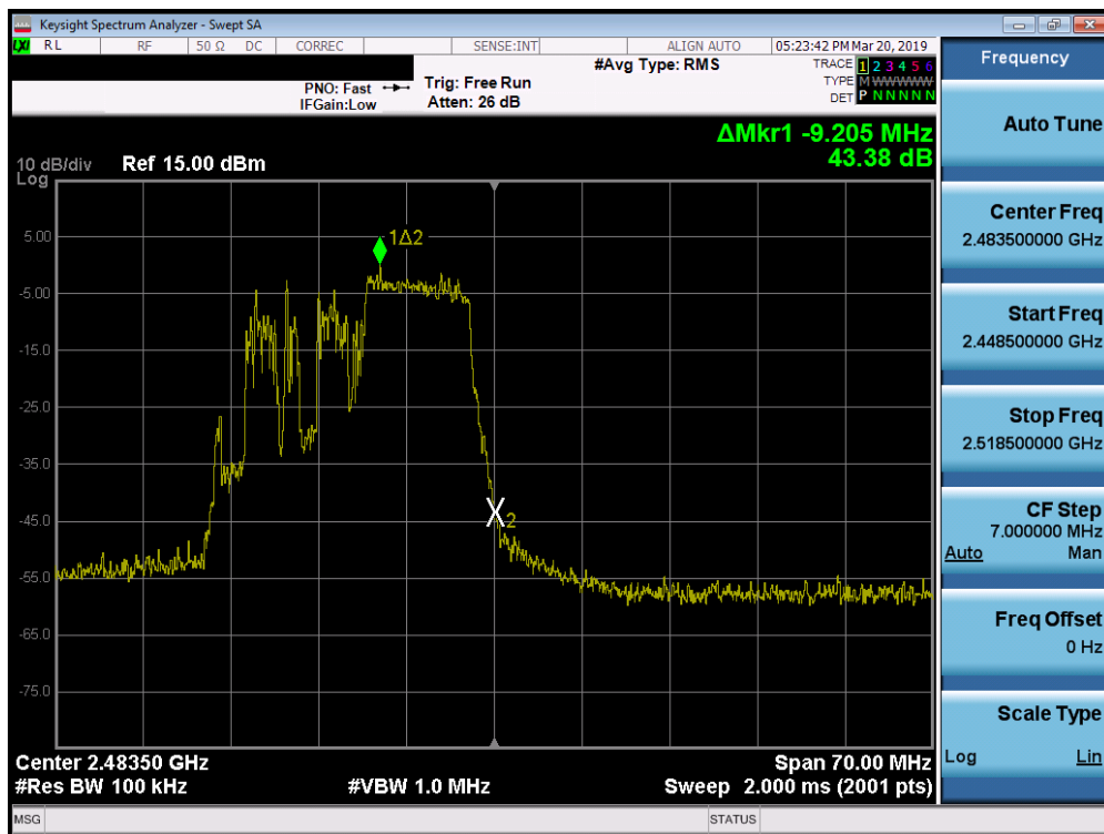
Plot 7-36. Band Edge Plot SISO ANT2 (802.11ax OFDMA – 106 Tones – Ch. 13)
