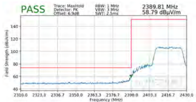
Plot 7-104. Radiated Restricted Lower Band Edge Measurement SISO ANT1 (Peak – 242 Tones)
