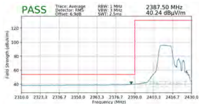
Plot 7-117. Radiated Restricted Lower Band Edge Measurement SISO ANT2 (Average – 106 Tones)
