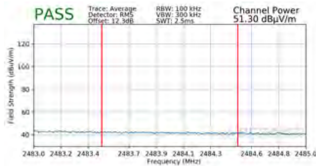
Plot 7-109. Radiated Restricted Upper Band Edge Measurement SISO ANT1 (Average – 242 Tones)
