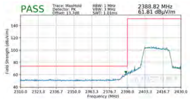
Plot 7-114. Radiated Restricted Band Edge Measurement SISO ANT1 with WCP (Peak – 242 Tones)
