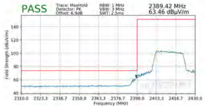
Plot 7-128. Radiated Restricted Lower Band Edge Measurement SISO ANT2 (Peak – 242 Tones)
