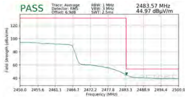
Plot 7-131. Radiated Restricted Upper Band Edge Measurement SISO ANT2 (Average – 242 Tones)
