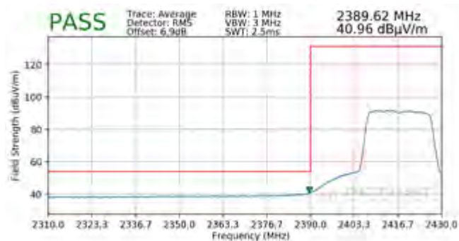
Plot 7-155. Radiated Restricted Lower Band Edge Measurement MIMO (Average – 242 Tones)
