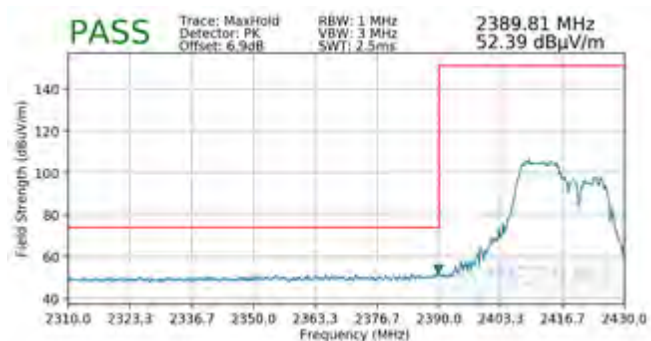
Plot 7-118. Radiated Restricted Lower Band Edge Measurement SISO ANT2 (Peak – 106 Tones)
