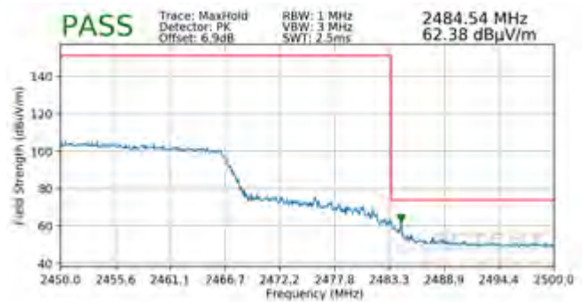
Plot 7-132. Radiated Restricted Upper Band Edge Measurement SISO ANT2 (Peak – 242 Tones)
