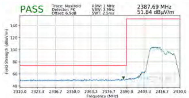
Plot 7-144. Radiated Restricted Lower Band Edge Measurement MIMO (Peak – 106 Tones)
