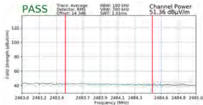
Plot 7-135. Radiated Restricted Upper Band Edge Measurement SISO ANT2 (Average – 242 Tones)
