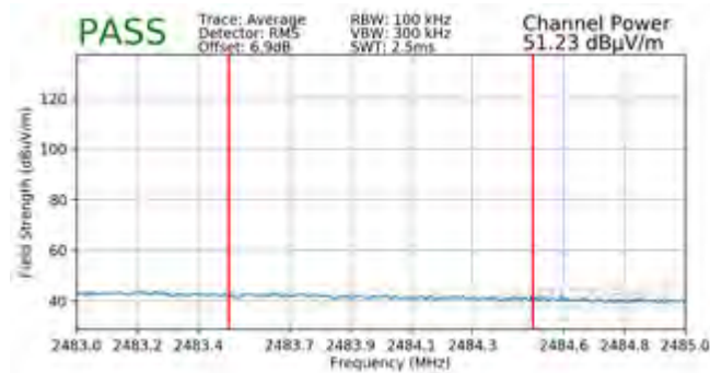
Plot 7-133. Radiated Restricted Upper Band Edge Measurement SISO ANT2 (Average – 242 Tones)
