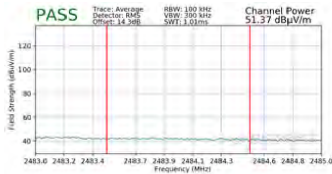
Plot 7-161. Radiated Restricted Upper Band Edge Measurement MIMO (Average – 242 Tones)
