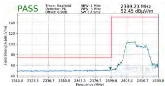
Plot 7-116. Radiated Restricted Lower Band Edge Measurement SISO ANT2 (Peak – 106 Tones)
