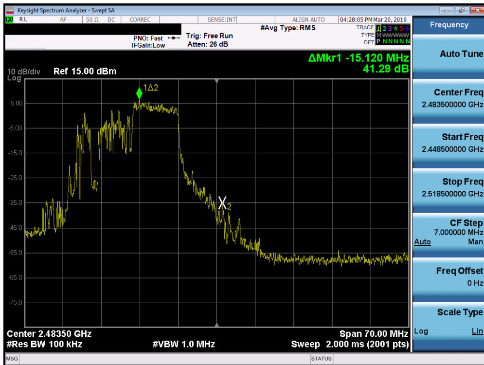
Plot 7-27. Band Edge Plot SISO ANT1 (802.11ax OFDMA - 106 Tones - Ch. 12)
