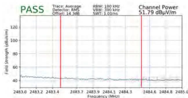
Plot 7-163. Radiated Restricted Upper Band Edge Measurement MIMO (Average – 242 Tones)
