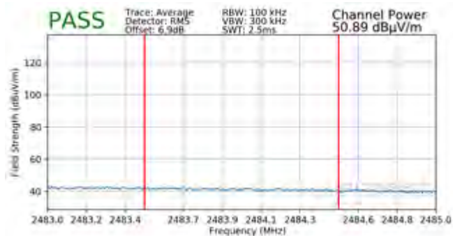
Plot 7-107. Radiated Restricted Upper Band Edge Measurement SISO ANT1 (Average – 242 Tones)
