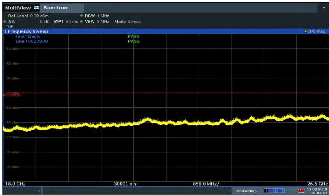
Plot 7-458. Radiated Spurious Plot 18GHz – 26.5GHz (Band 30 – H - OPEN)
