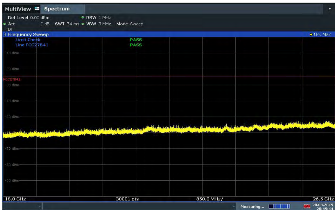
Plot 7-469. Radiated Spurious Plot 18GHz – 26.5GHz (Band 41 PC2 – V - CLOSED)
