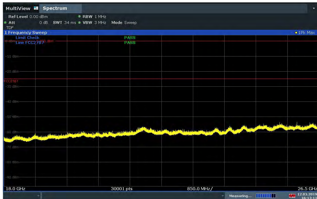
Plot 7-465. Radiated Spurious Plot 18GHz – 26.5GHz (Band 7 – V - OPEN)
