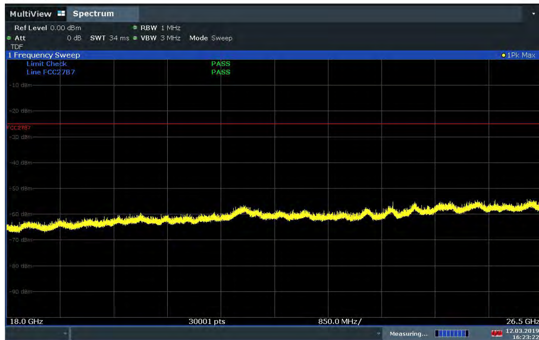
Plot 7-464. Radiated Spurious Plot 18GHz – 26.5GHz (Band 7 – H - OPEN)
