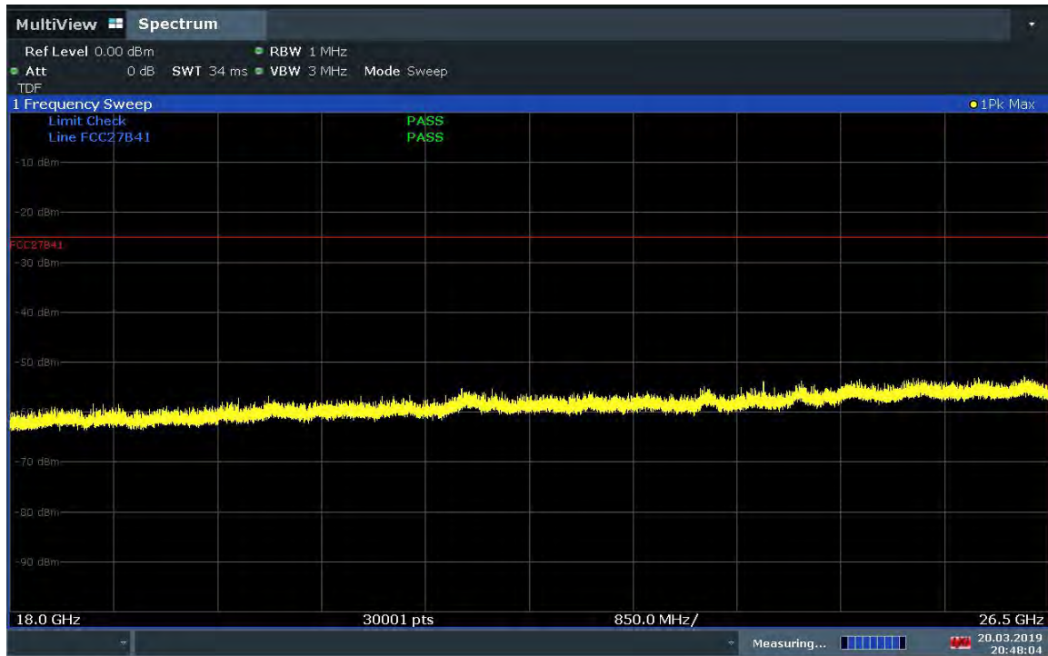
Plot 7-468. Radiated Spurious Plot 18GHz – 26.5GHz (Band 41 PC2 – H - CLOSED)
