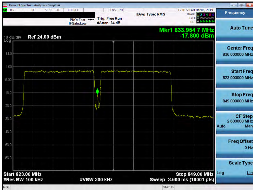
Plot 7-413. Conducted Spurious Plot (Band 5B – 10.0MHz QPSK – PCC 50/0 SCC 50/0 – Low Channel)
