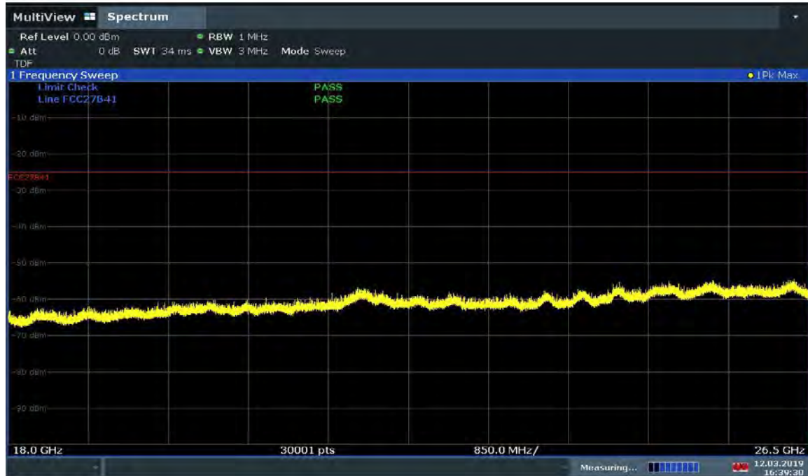
Plot 7-471. Radiated Spurious Plot 18GHz – 26.5GHz (Band 41 PC2 – V - OPEN)
