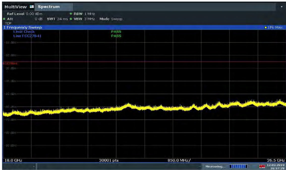
Plot 7-470. Radiated Spurious Plot 18GHz – 26.5GHz (Band 41 PC2 – H - OPEN)
