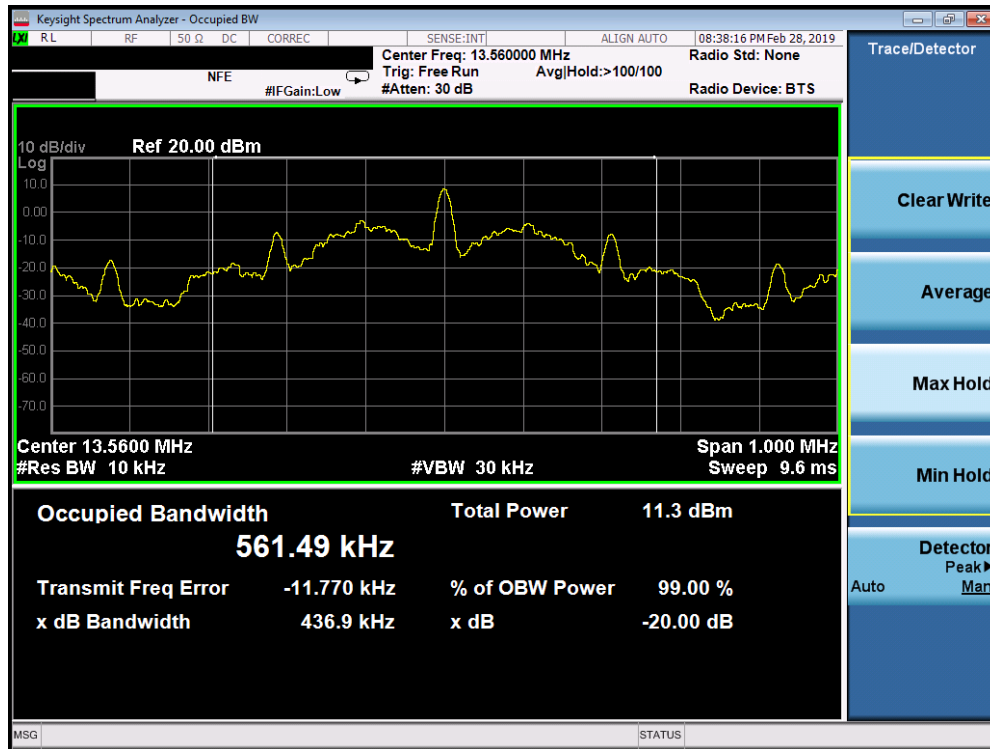
Figure 7-2. Occupied Bandwidth Plot
