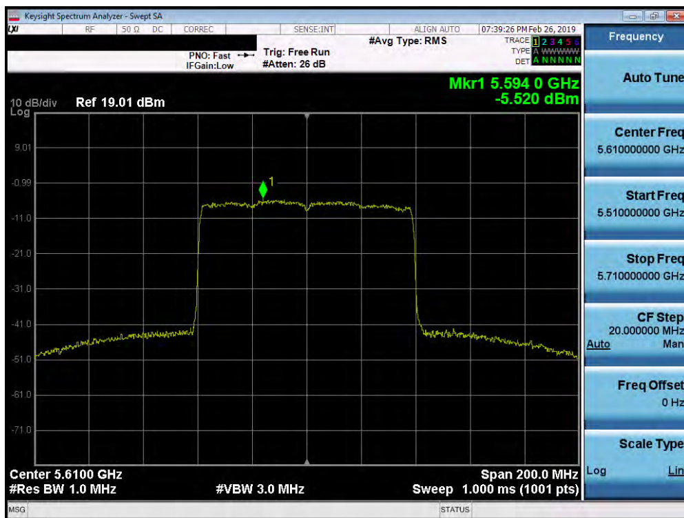
Plot 7-182. Power Spectral Density Plot SISO ANT1 (80MHz BW 802.11ax (UNII Band 2C) – Ch. 122)
