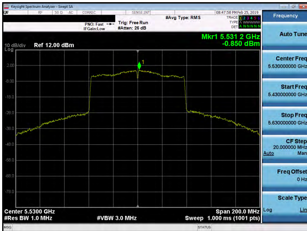
Plot 7-178. Power Spectral Density Plot SISO ANT1 (80MHz BW 802.11ac (UNII Band 2C) – Ch. 106)
