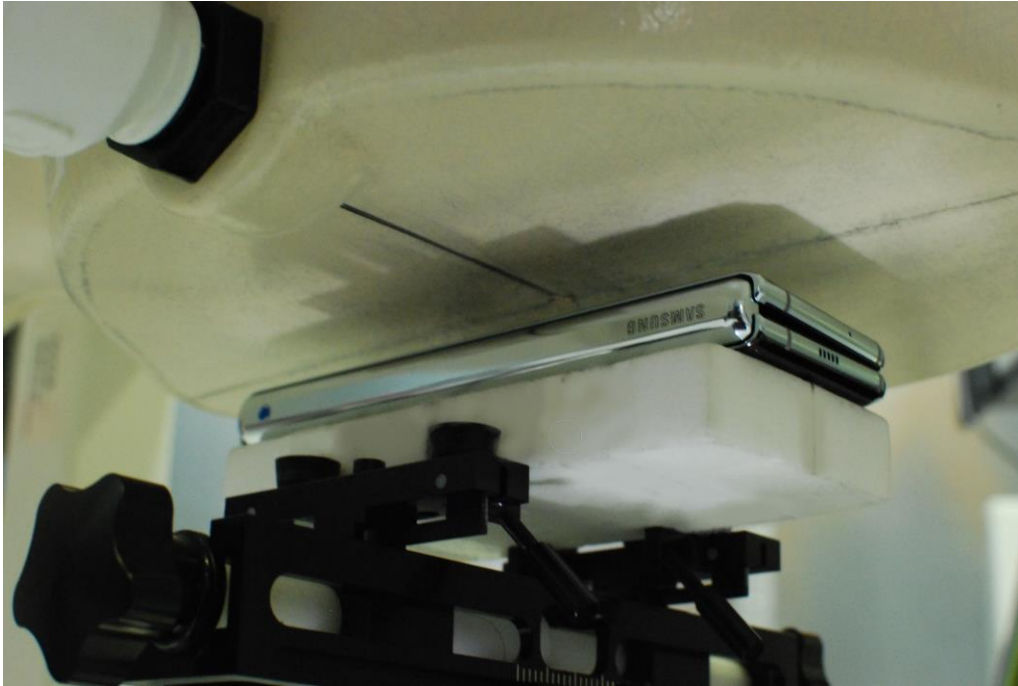
SAR Test Setup Photo 5 – Closed Configuration Back Side at 1.5cm
