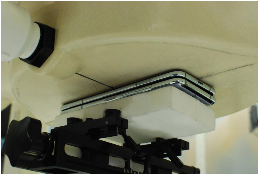
SAR Test Setup Photo 10 – Closed Configuration Front Side at 0.0cm
